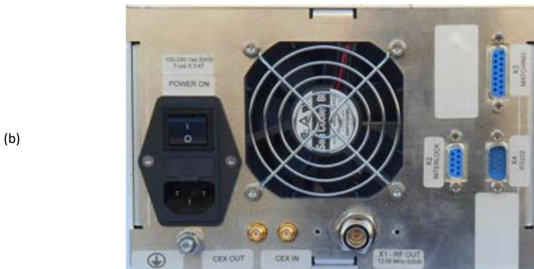
Figura 18. Active Front Panel (a) del RF generator a 200 W (b).
