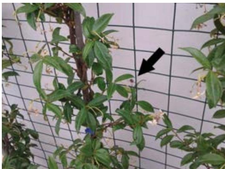
Figure 2. Sensor for the measurement of the surface temperature of the external plaster
