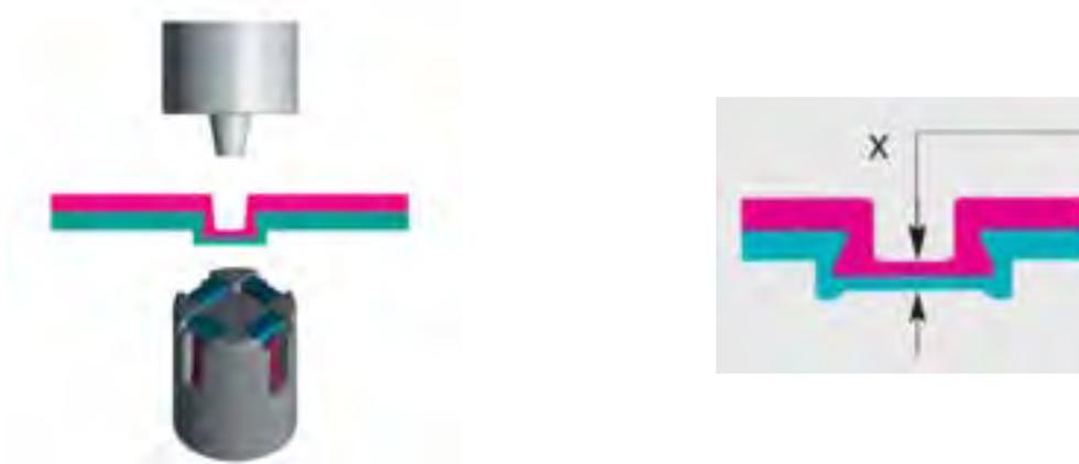
**Figura 57: SET matrice a setti mobili - punzone TOX SBK**
