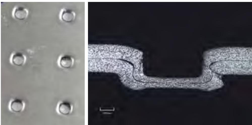
Figura 60: SET matrice a setti mobili - punzone TOX SBK
