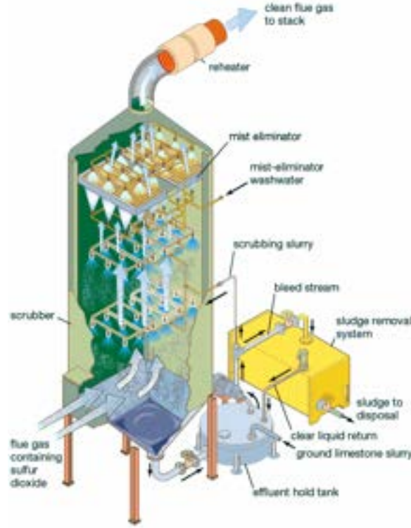
Figure 3.1: Flue gas desulfurization limestone wet scrubber [3.7]
