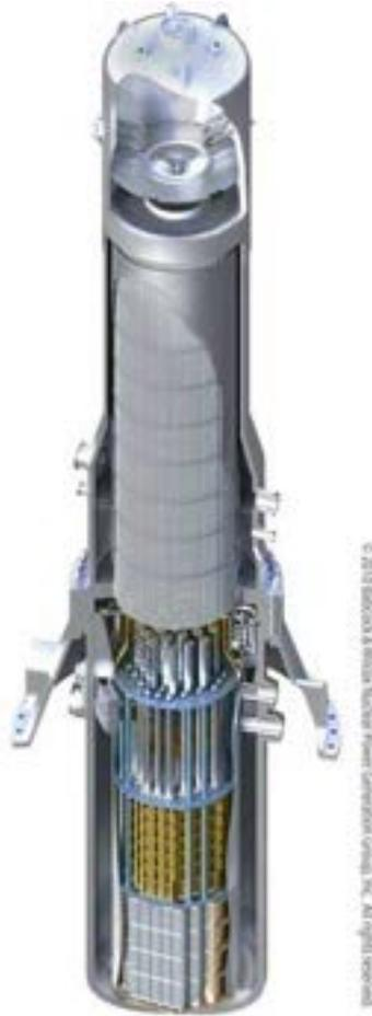
Figure 3.2.1 mPower reactor core
