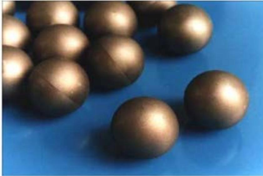
Figure 3.14.2 Spherical fuel elements
