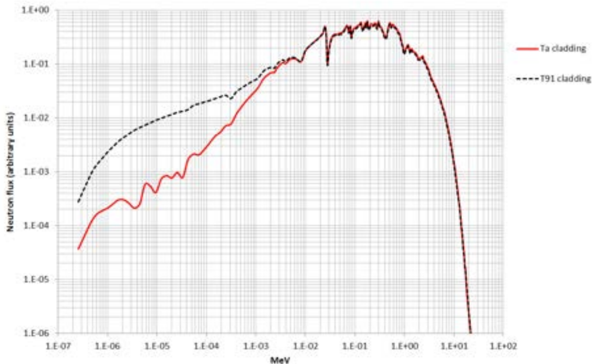
Figure 4. Neutron spectrum in the T91 and Ta cladding in the outer core zone.
