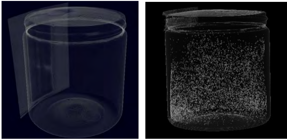
Figure 12. Computed tomography scans of a superheated emulsion of C-318 after an irradiation with 1 gray of 6 MV X-rays (left) and after an irradiation with 250 mrem of Am-Be neutrons (right) . The neutron irradiation was delivered using two sources in contact with opposite sides of the detector.
