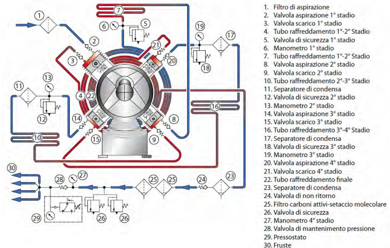
**Figura 10:** MCH-30 Silent: circuito in pressione
