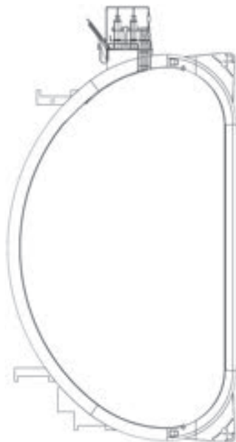
Figure 11.1 – Orientation of Coil for Shipping (Top view)
