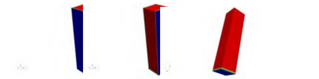
Figure 2.21: Boundary conditions for the velocity components u , v (center and left) and w and temperature field ( T ) (both in right). The blue color indicates the type of boundary conditions Dirichlet ; the red boundary conditions of type Neumann .
