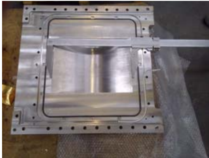
Fig. 19 Dimensional check of the Backplate
