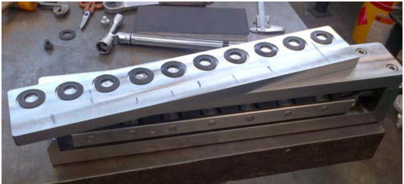
fig. 20 frame mock-up with Belleville springs
