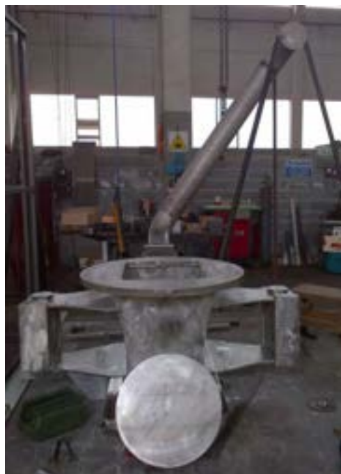
fig. 14 TA body welding (inlet pipe positioning)
