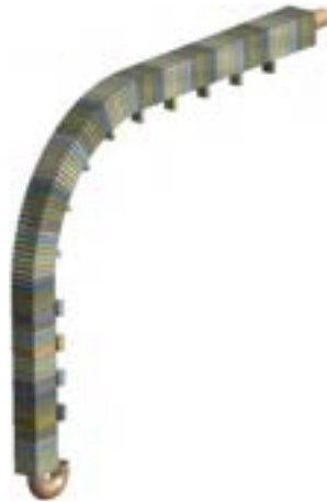
Figure 2. Plasma facing unit of the OVT geometry.
