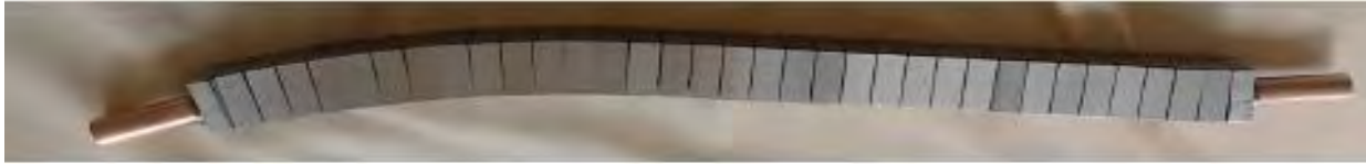
Fig. 3 Actively cooled tungsten monoblocks mock up
