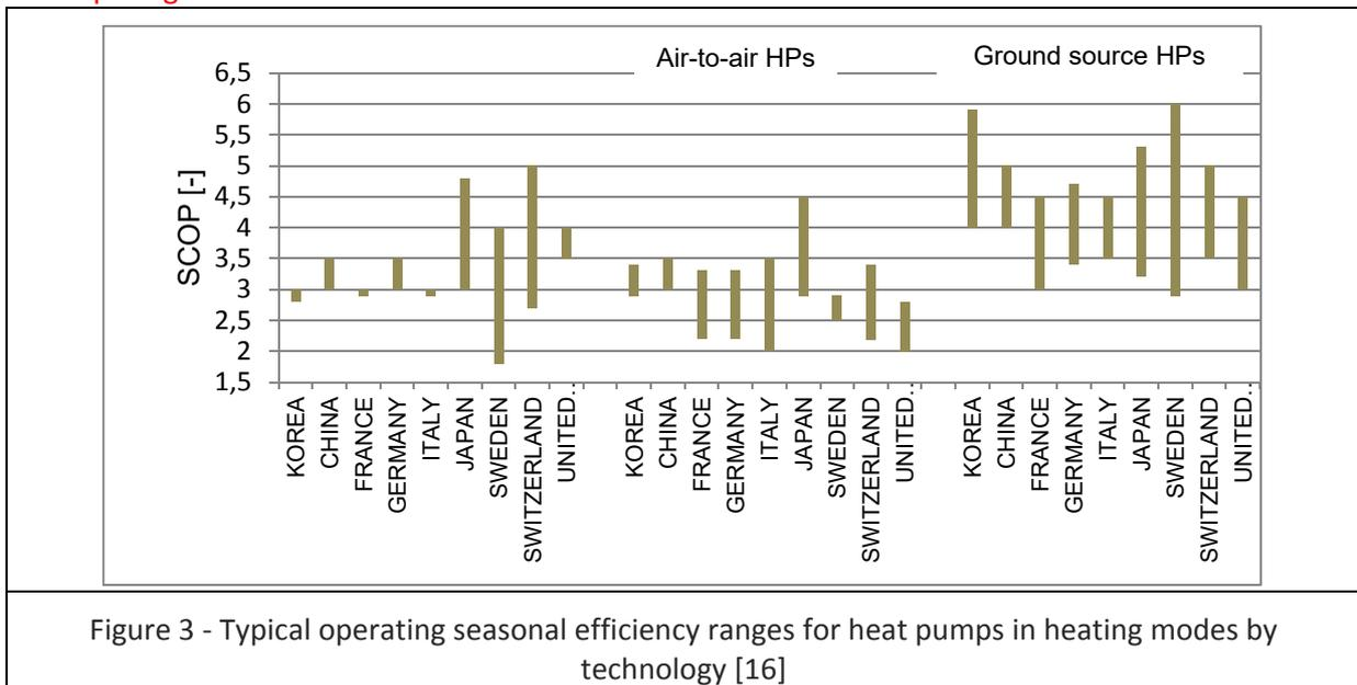
Figure 3 - Typical operating seasonal efficiency ranges for heat pumps in heating modes by technology [16]
