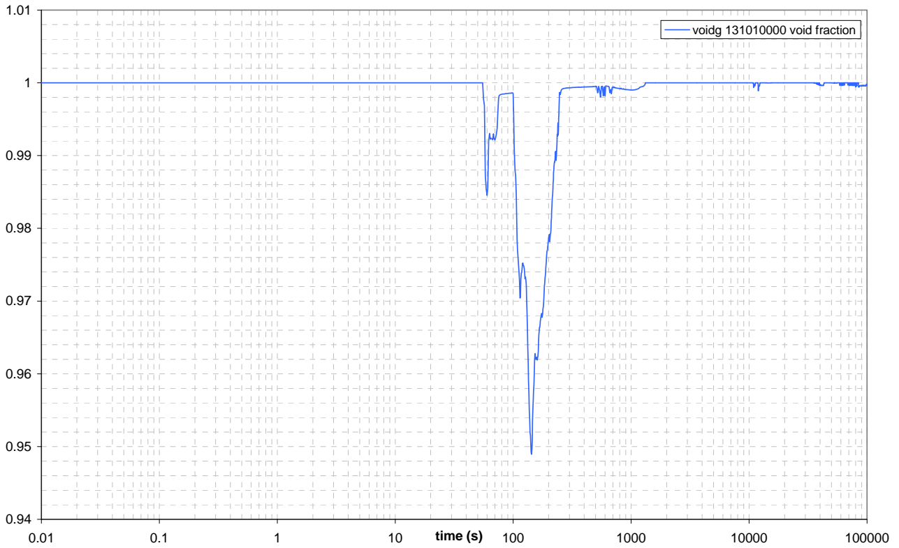
Figure 5.53: EBT TEST, ADS DT (Stage-I) LINE void fraction DOWNSTREAM
