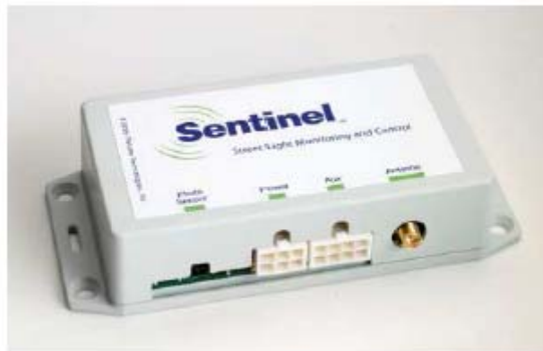
Figura 83 Wireless Lighting Control
