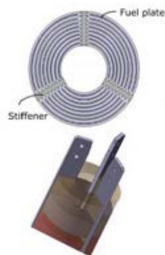
Figure 2) JHR fuel element
