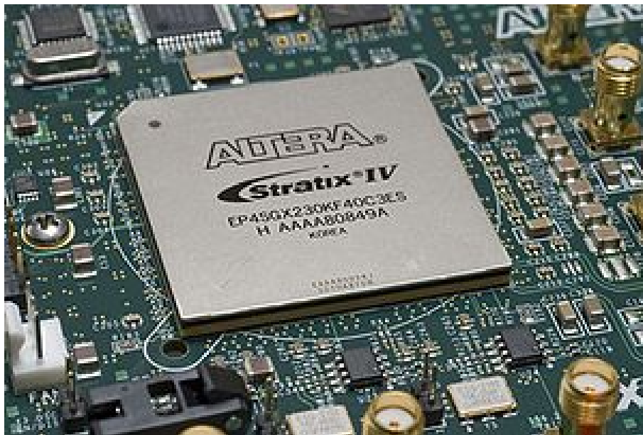
Figure 7: Example of an FPGA-based application
