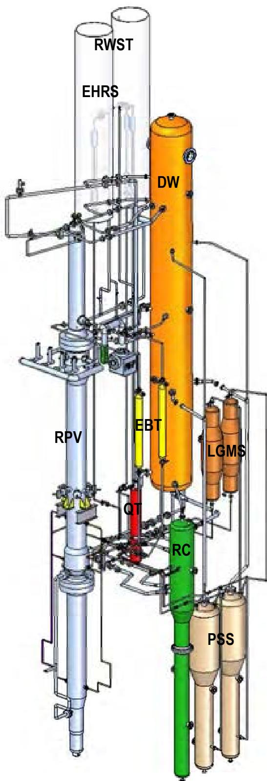
Fig.3. 2 – SPES3 primary, secondary loop B, and containment system layout
