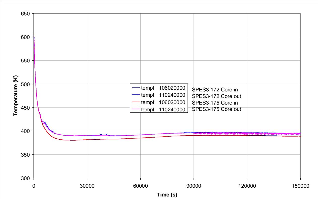
**Fig.7. 62 - SPES3-172 and SPES3-175 Core heater rod surface temperature –normal rod (window)**
