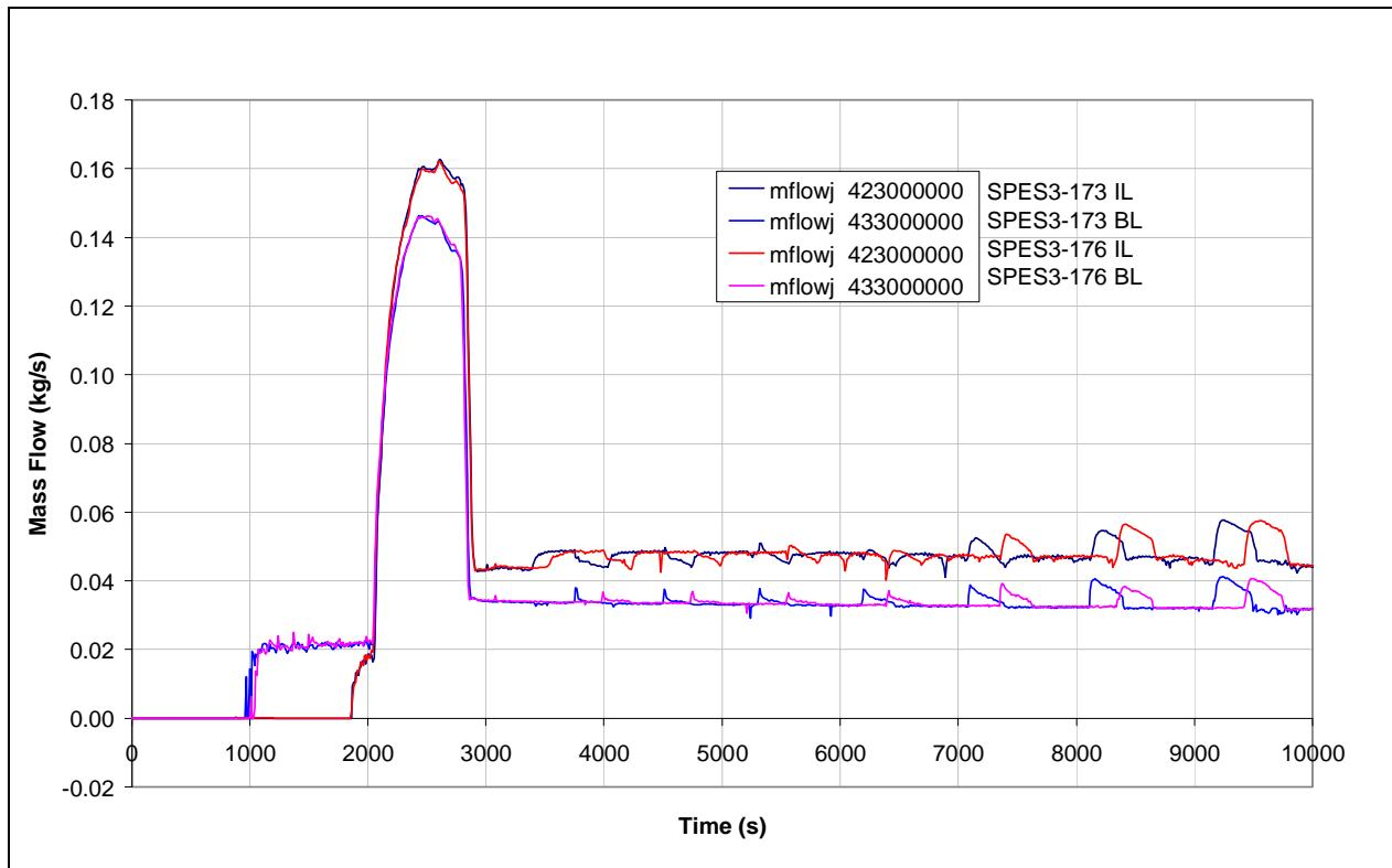
**Fig.8. 6 – SPES3-173 and SPES3-176 LGMS injection mass flow**
