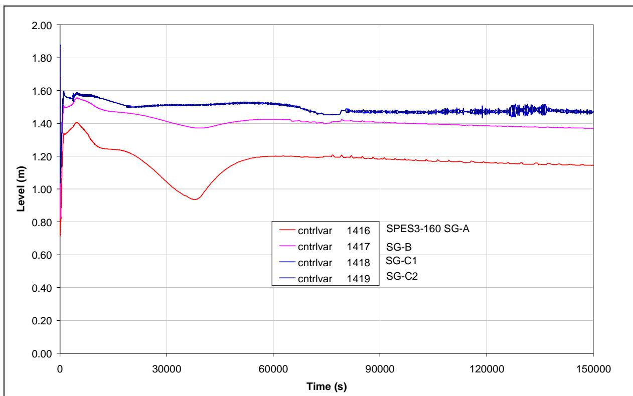
**Fig.4.45 – SPES3-160 PRZ level**
