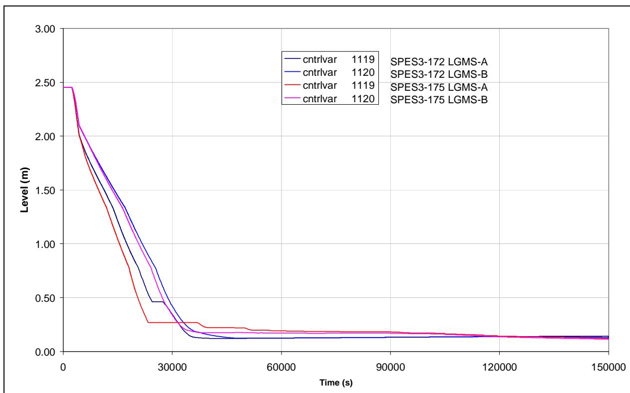
**Fig.7. 67 - SPES3-172 and SPES3-175 DW level**
