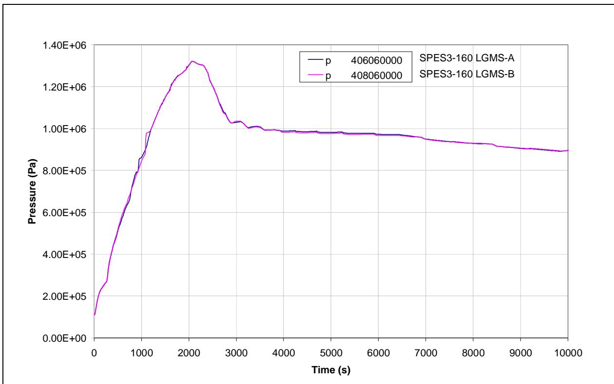
**Fig.4.22 – SPES3-160 LGMS pressure**
