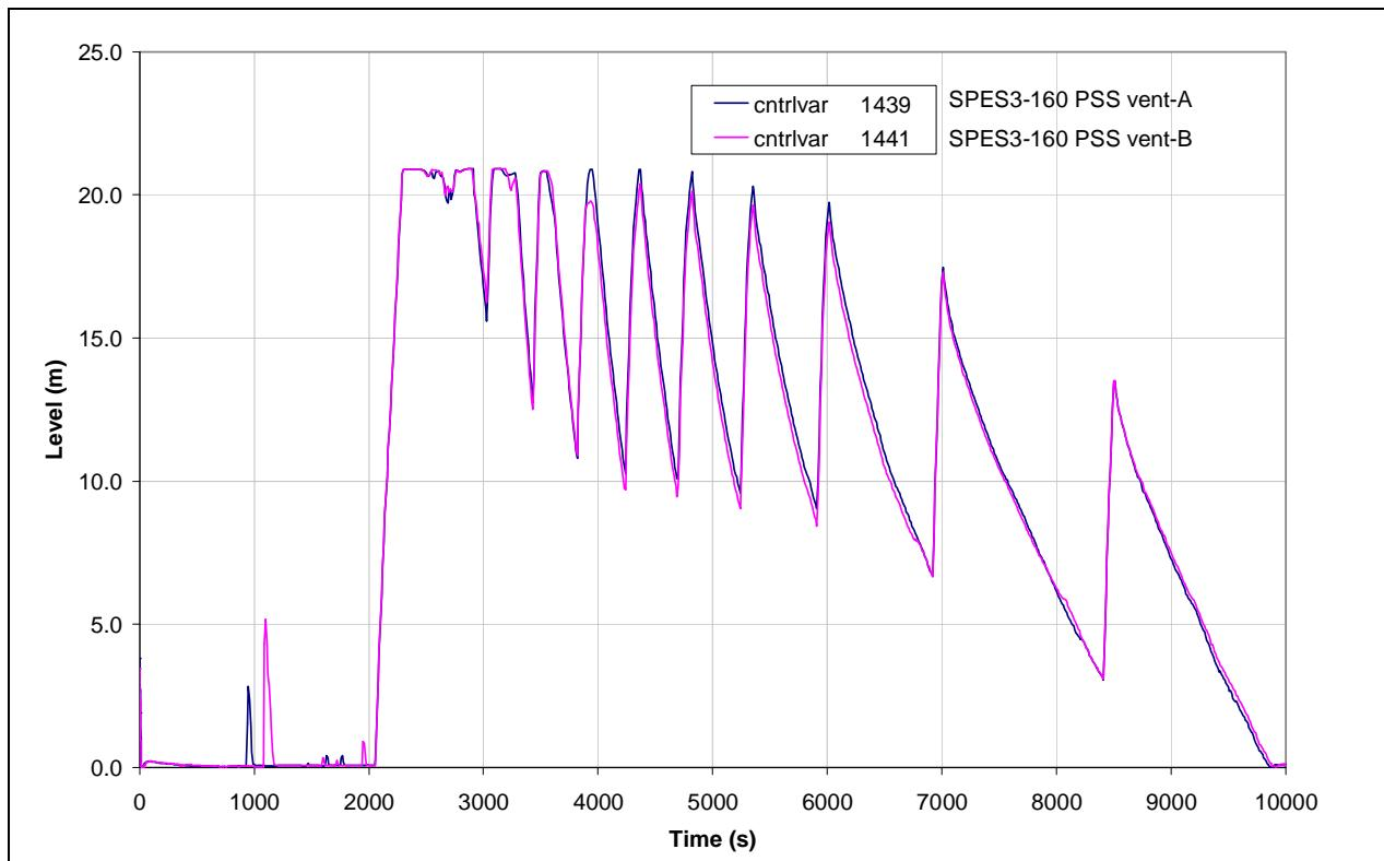
**Fig.4.26 – SPES3-160 PSS vent pipe level**
