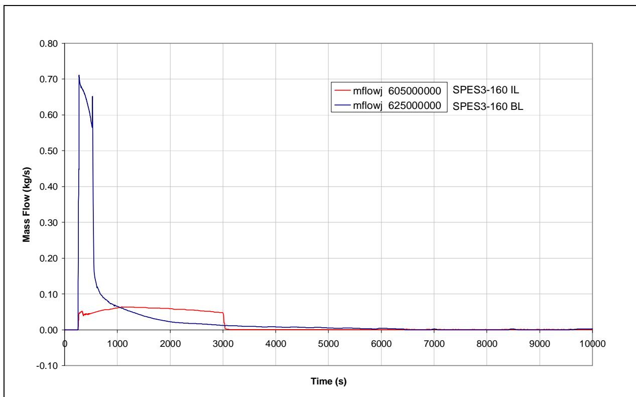
**Fig.4.4 – SPES3-160 LGMS injection mass flow**
