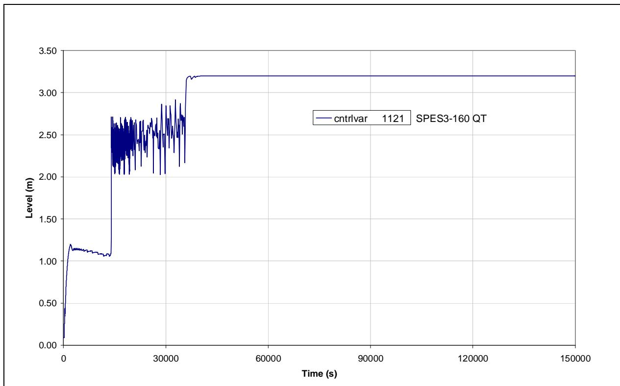
**Fig.4.33 – SPES3-160 LGMS level**
