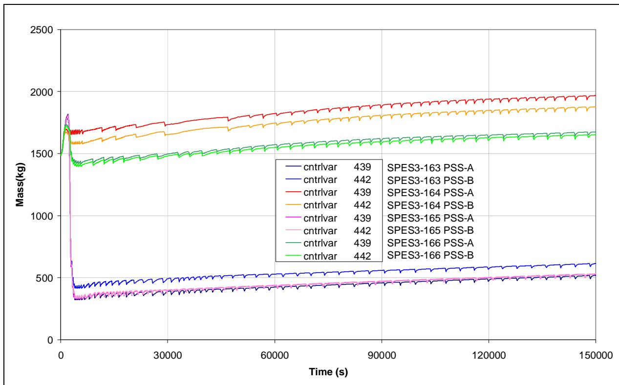
**Fig.5. 22 – SPES3-163, 164, 165 and 166 LGMS-A mass (intact loop)**
