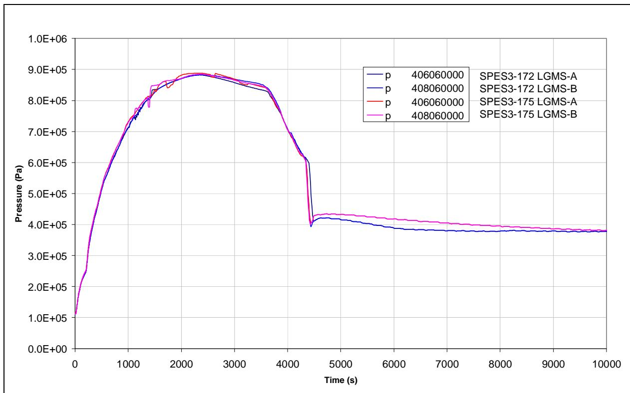
**Fig.7. 25 - SPES3-172 and SPES3-175 LGMS pressure**
