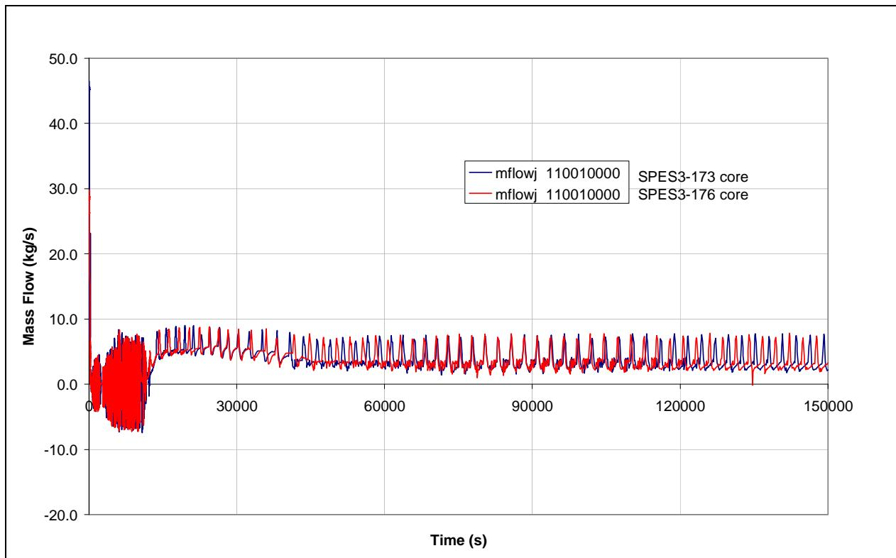
**Fig.8. 58 – SPES3-173 and SPES3-176 RI-DC check valve mass flow (window)**
