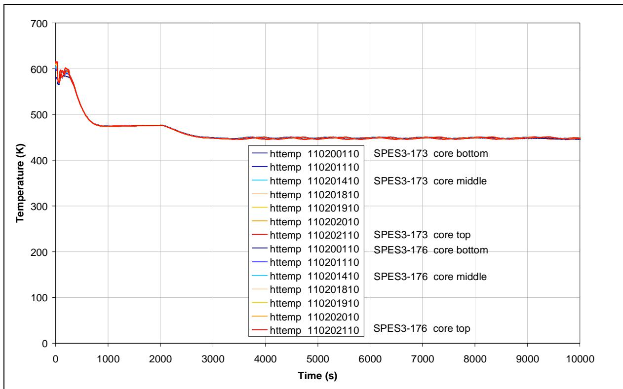
**Fig.8. 74 – SPES3-173 and SPES3-176 Core heater rod clad surface temperatures (hot rods)**
