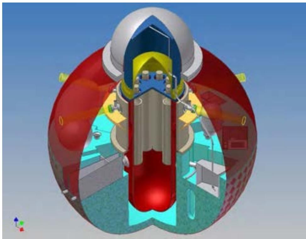
**Fig.3. 9 – IRIS Engineered Safety Feature scheme**
