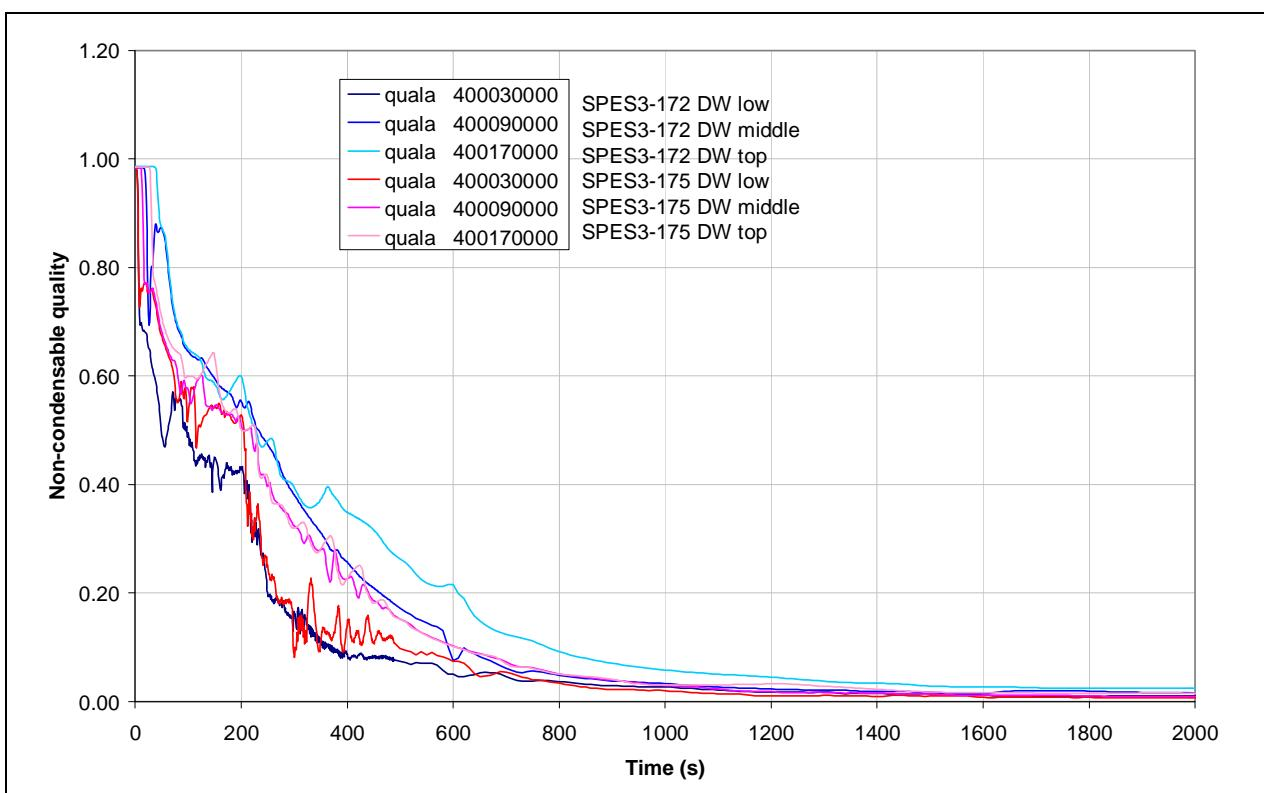
**Fig.7. 21 - SPES3-172 and SPES3-175 DW non-condensable gas quality**
