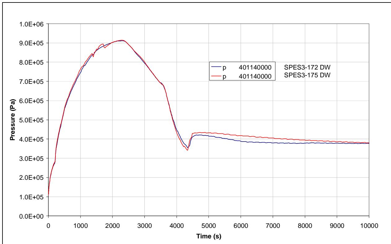
**Fig.7. 12 - SPES3-172 and SPES3-175 DW pressure**
