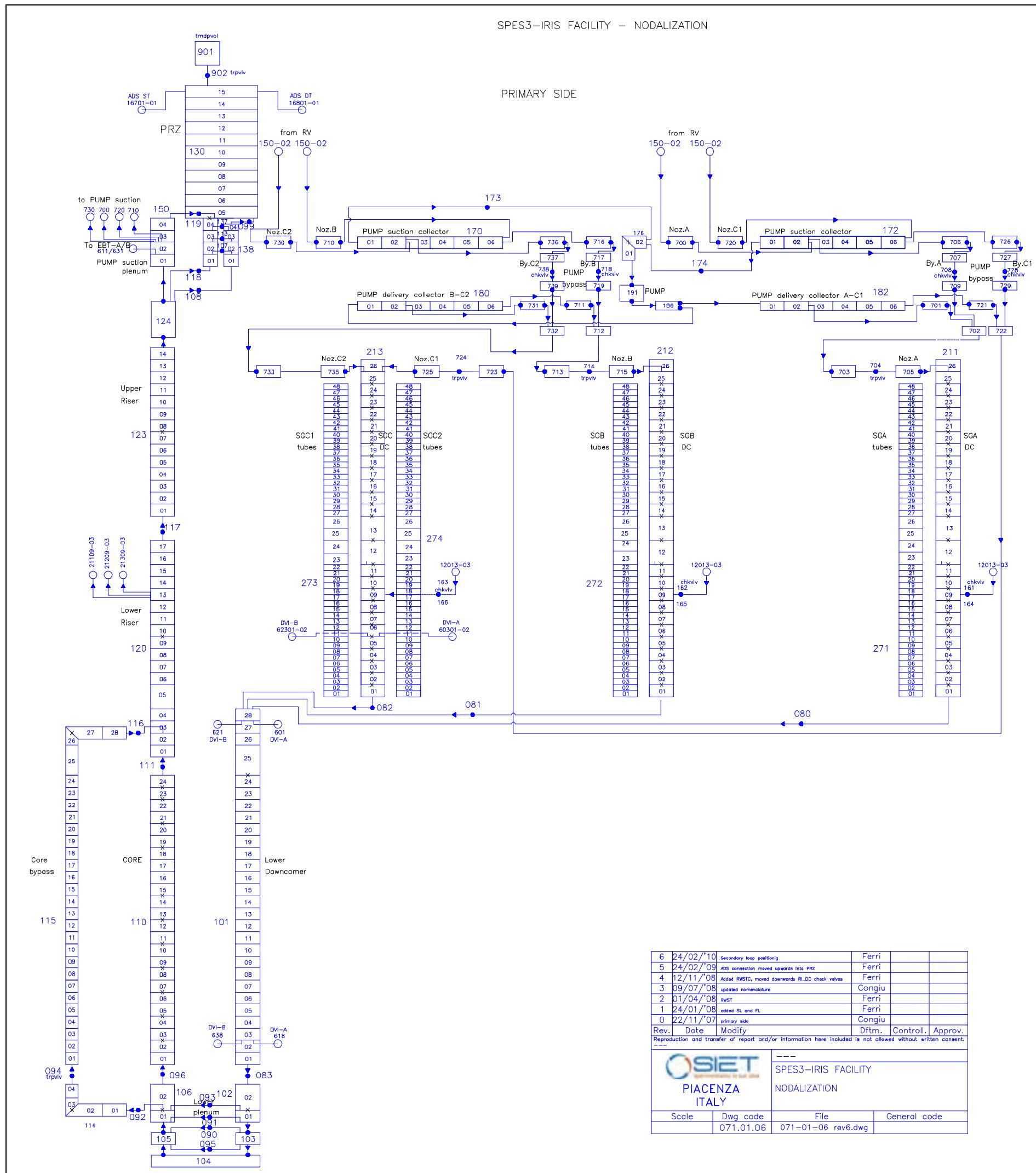
Fig.3. 5 – SPES3 Secondary Systems and EHRSs RELAP5 nodalization
