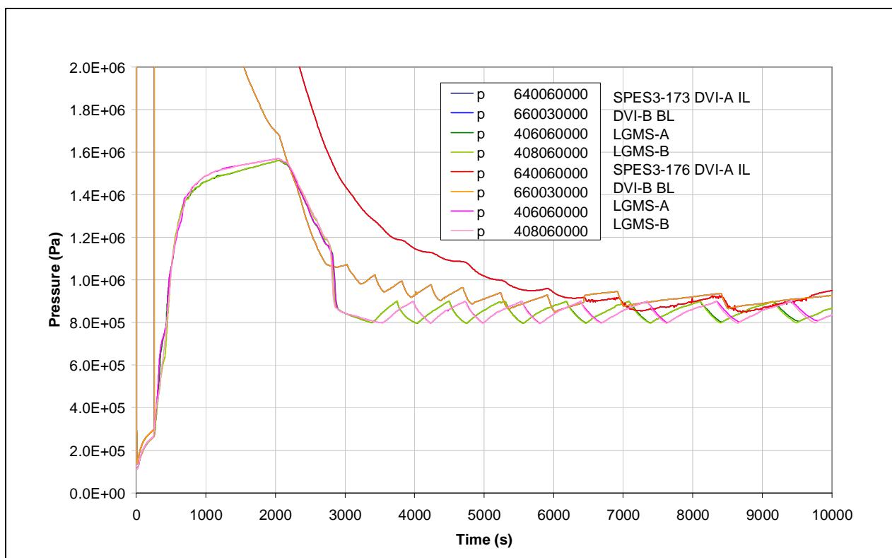
**Fig.8. 83 – SPES3-173 and SPES3-176 LGMS and DVI pressure (window)**
