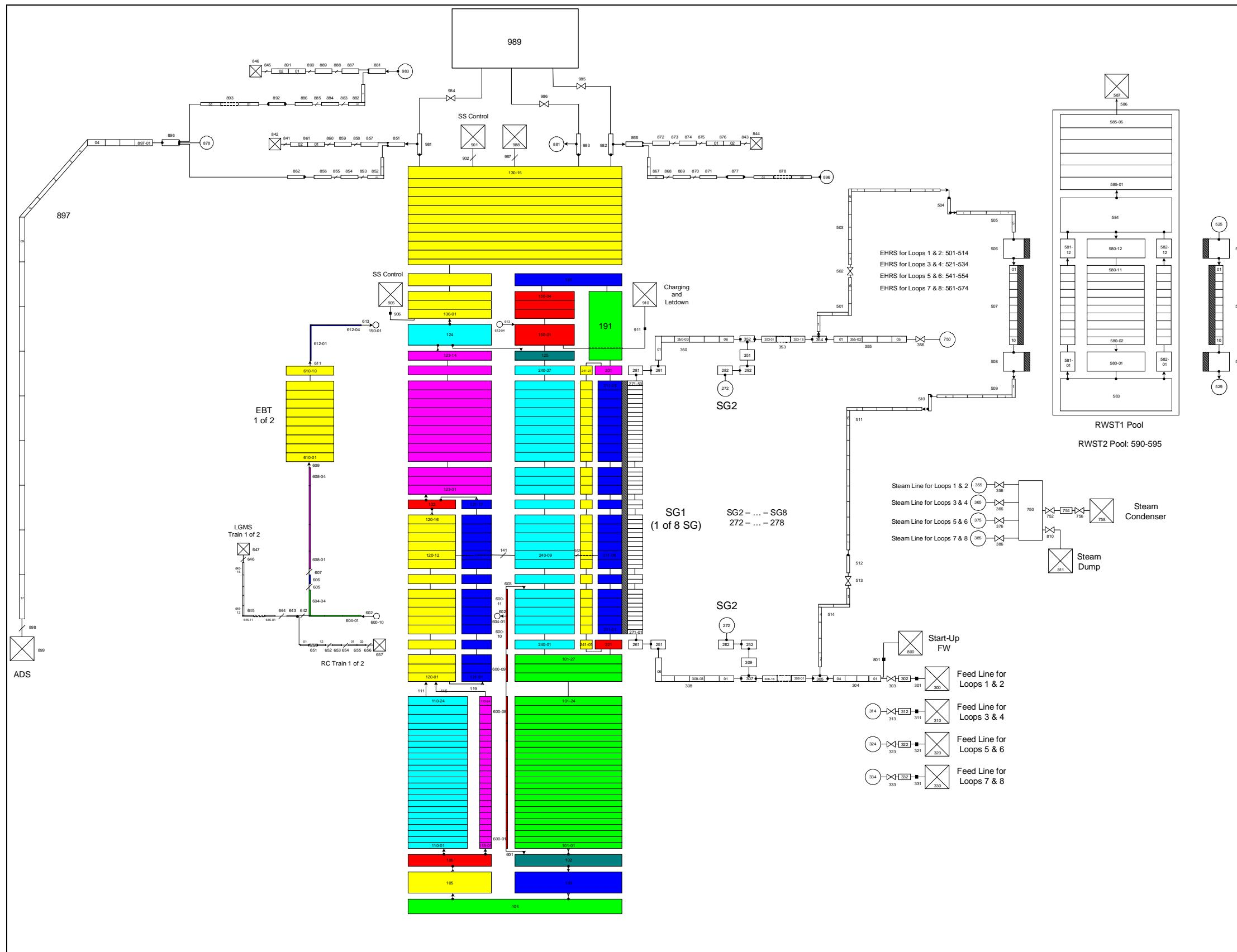
**Fig.3. 11 – IRIS Containment system GOTHIC**
