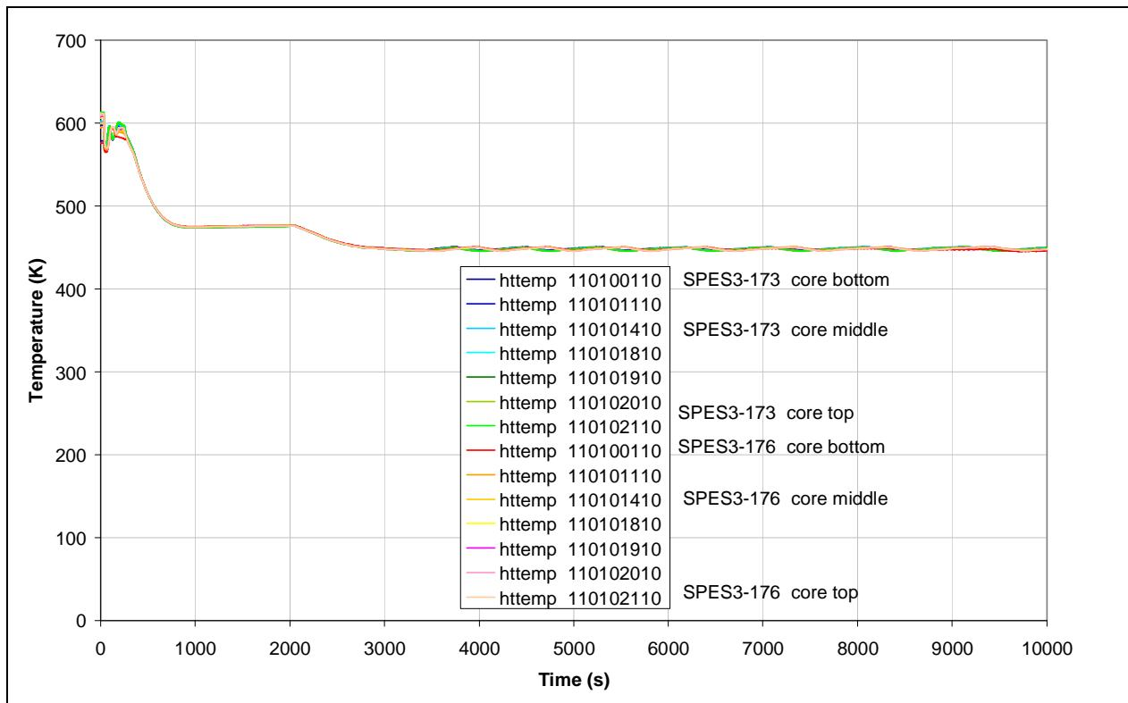
**Fig.8. 72 – SPES3-173 and SPES3-176 Core heater rod clad surface temperatures (normal rods)**
