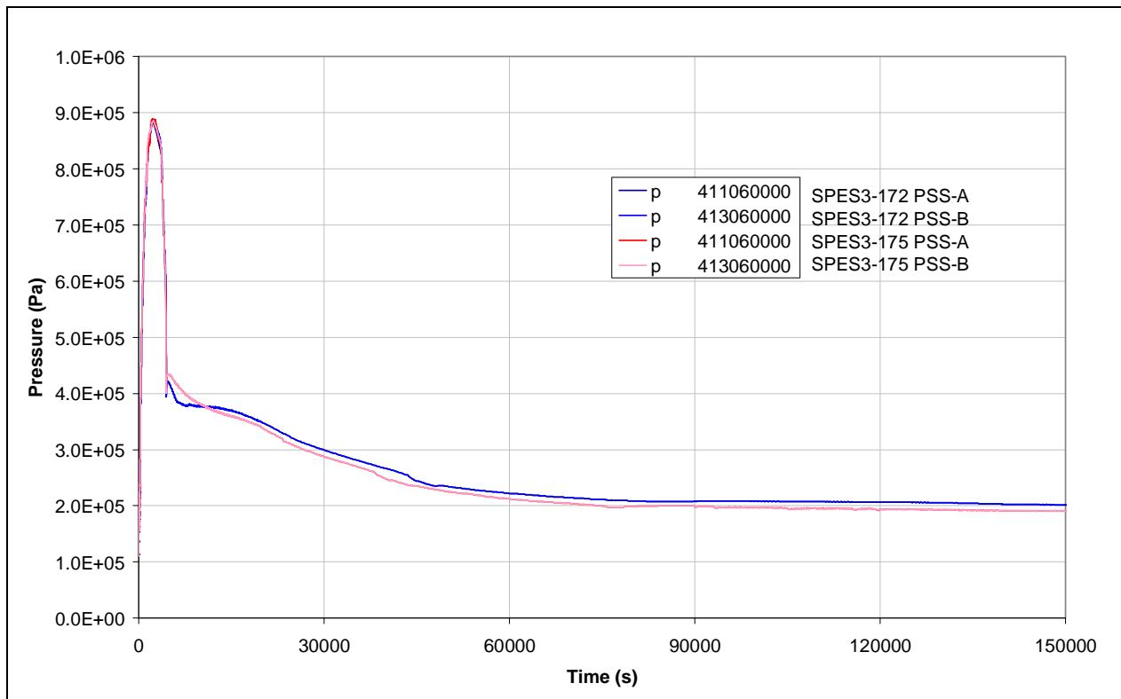
**Fig.7. 24 - SPES3-172 and SPES3-175 LGMS pressure (window)**
