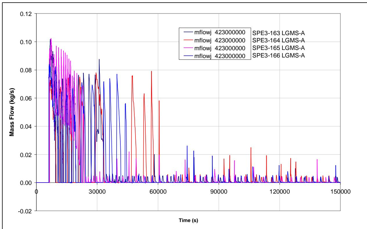
**Fig.5. 24 – SPES3-163, 164, 165 and 166 RC to DVI line mass flow (intact loop)**
