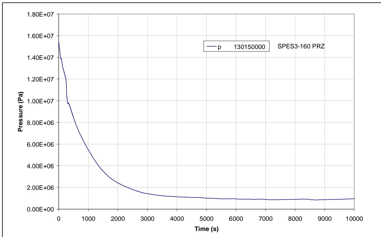
**Fig.4.8 – SPES3-160 PRZ pressure**
