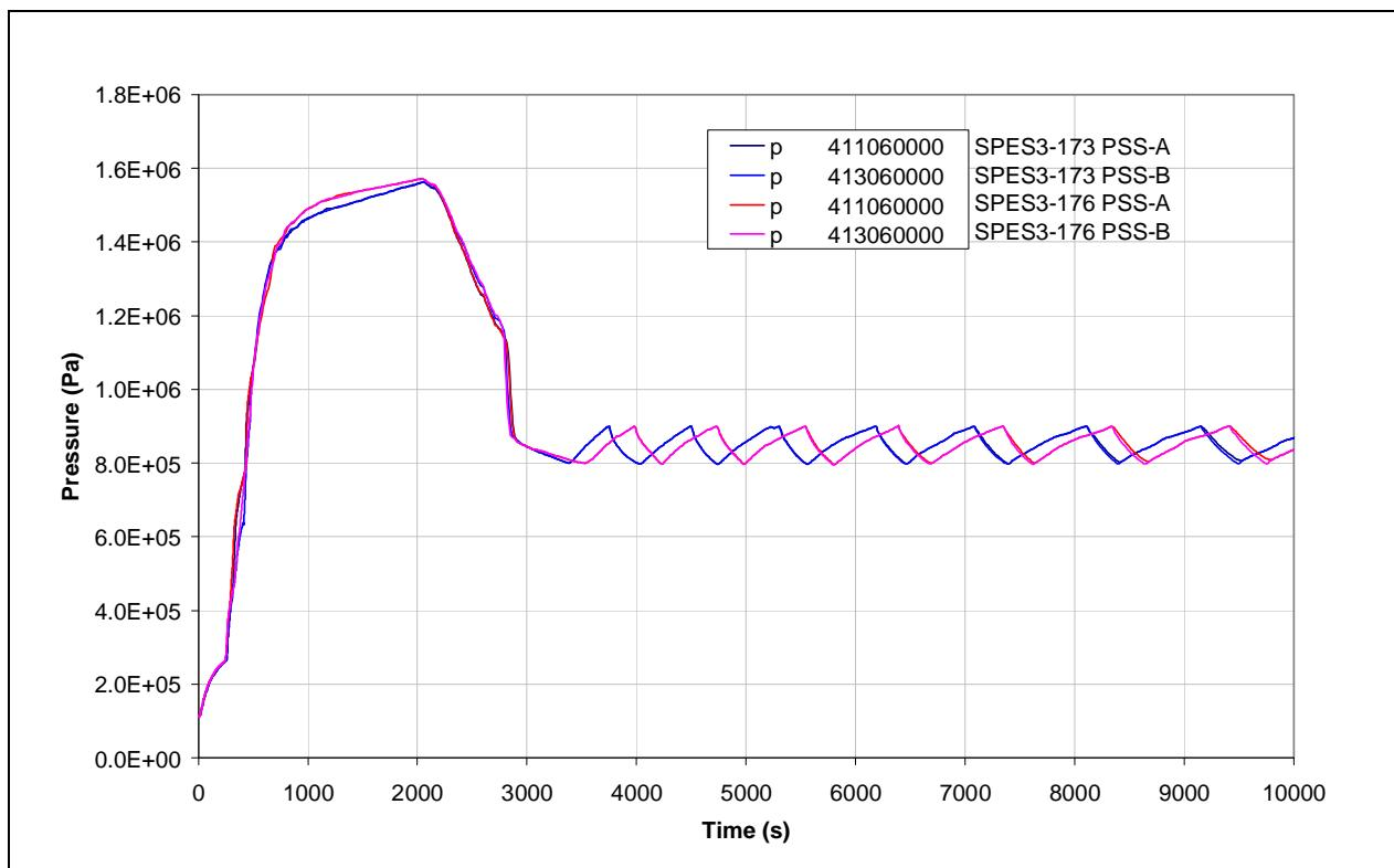
**Fig.8. 27 – SPES3-173 and SPES3-176 PSS pressure**
