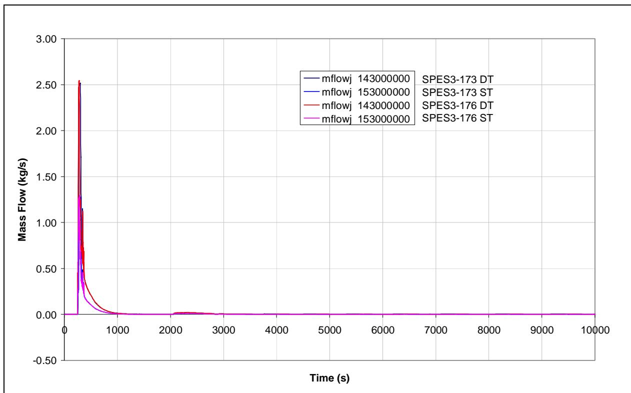
**Fig.8. 9 – SPES3-173 and SPES3-176 ADS Stage-II mass flow (window)**
