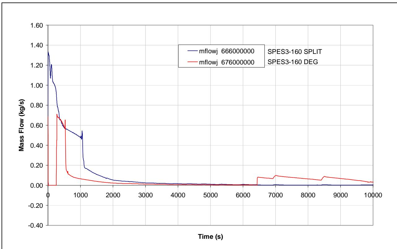
**Fig.4.2 – SPES3-160 DVI line break flow**
