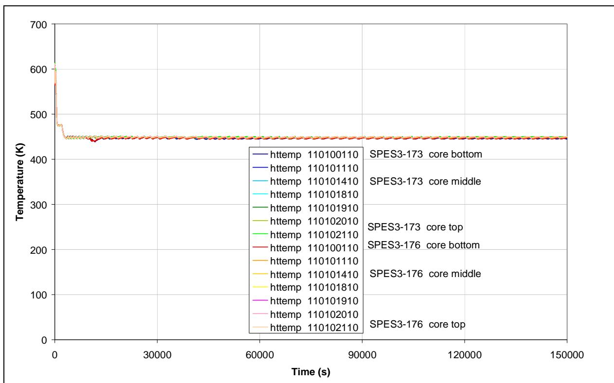
**Fig.8. 73 – SPES3-173 and SPES3-176 Core heater rod clad surface temperatures (hot rods) (window)**
