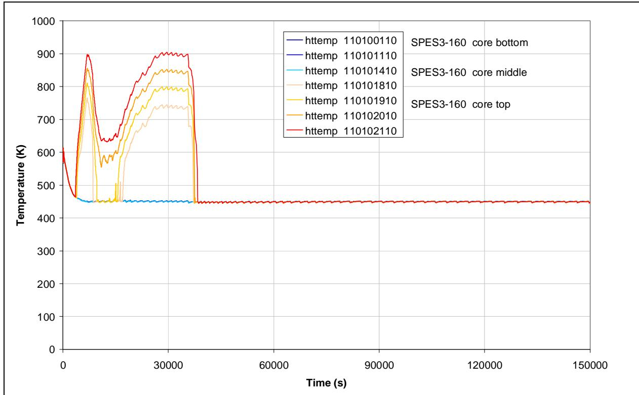
**Fig.4.60 – SPES3-160 Core heater rod clad surface temperatures (hot rods)**
