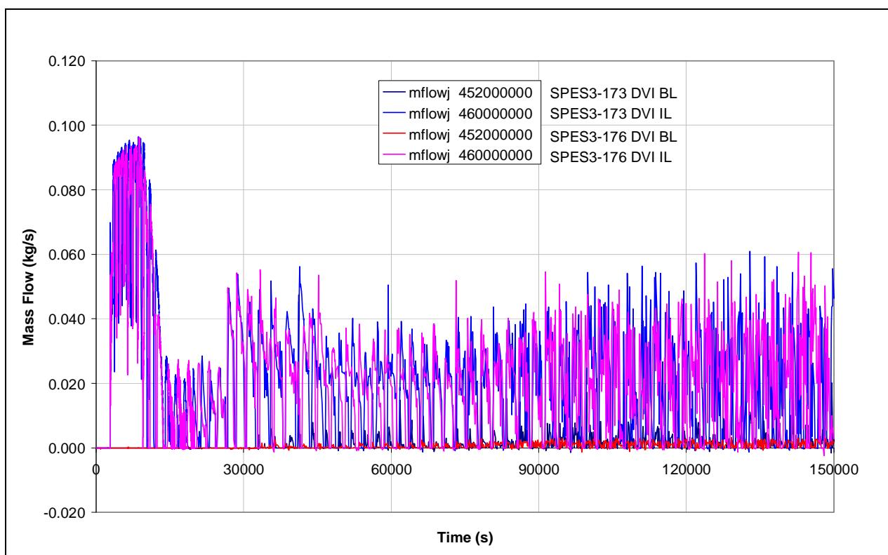
**Fig.8. 67 – SPES3-173 and SPES3-176 DVI line mass flow (window)**
