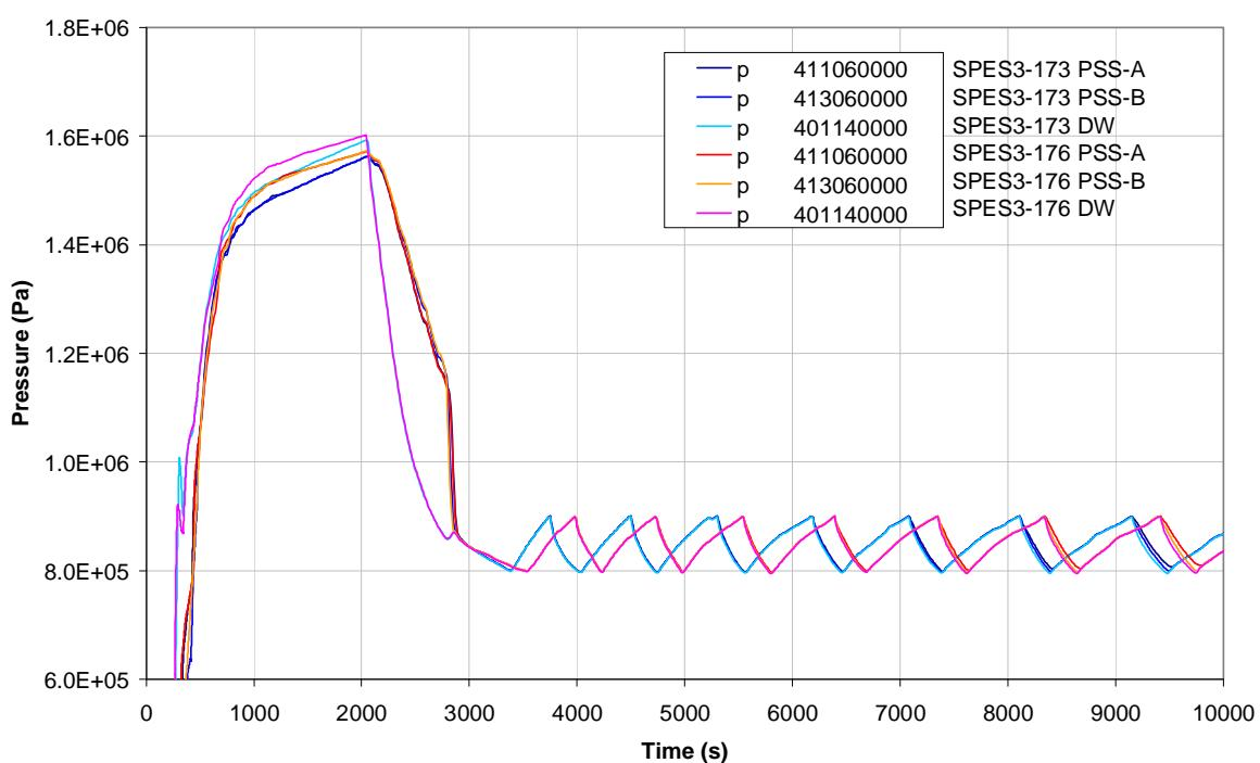
**Fig.8. 31 – SPES3-173 and SPES3-176 PSS and DW pressure**
