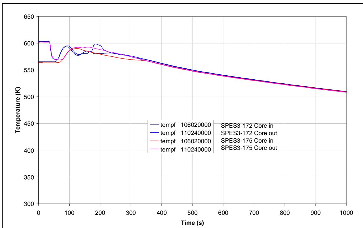
**Fig.7. 61 - SPES3-172 and SPES3-175 Core inlet and outlet fluid temperature**
