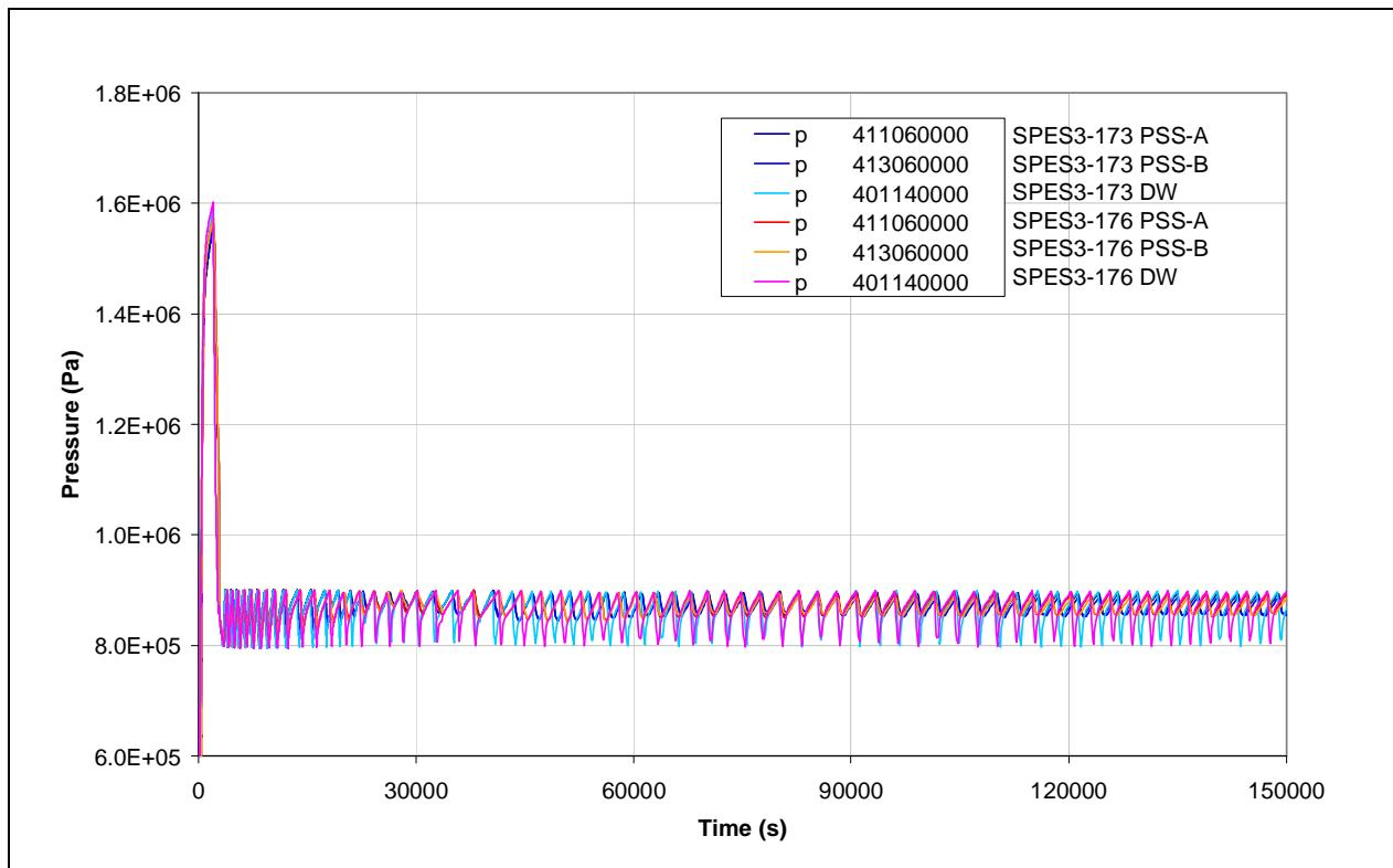
**Fig.8. 32 – SPES3-173 and SPES3-176 PSS vent pipe level (window)**
