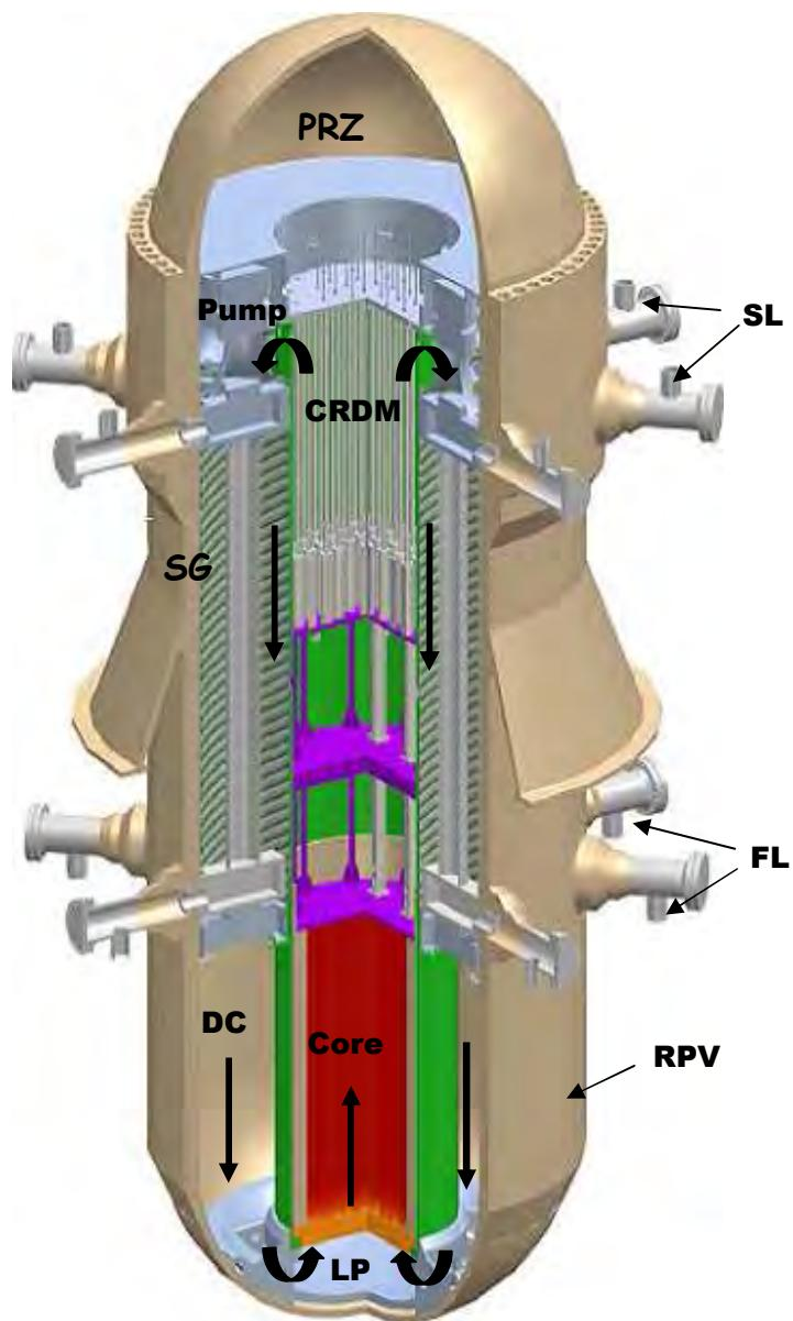
**Fig.3. 8 – IRIS Containment System general view**
