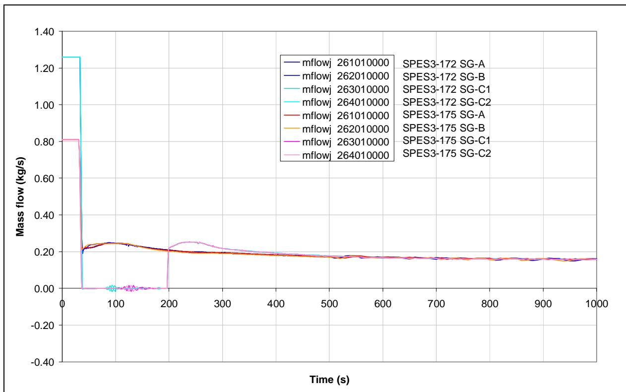
**Fig.7. 36 - SPES3-172 and SPES3-175 SG ss mass flow**
