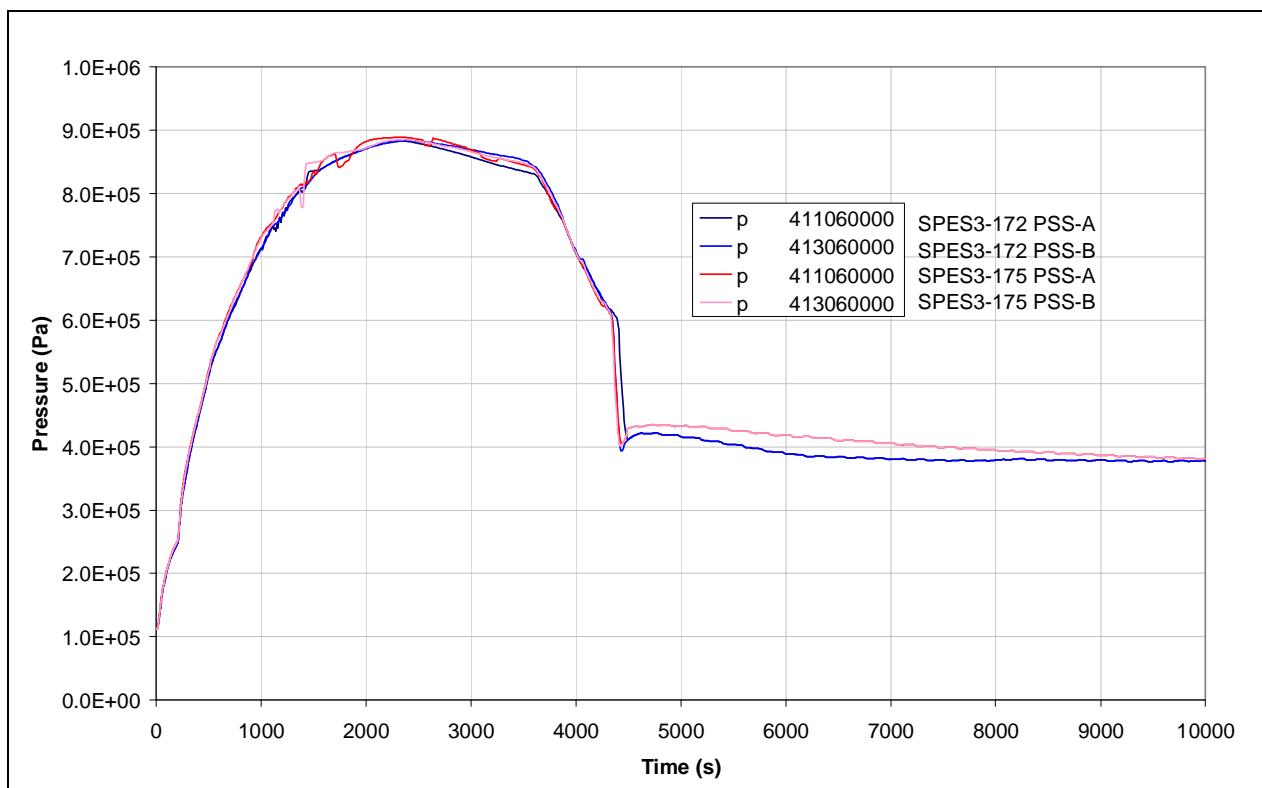
**Fig.7. 23 - SPES3-172 and SPES3-175 PSS pressure**
