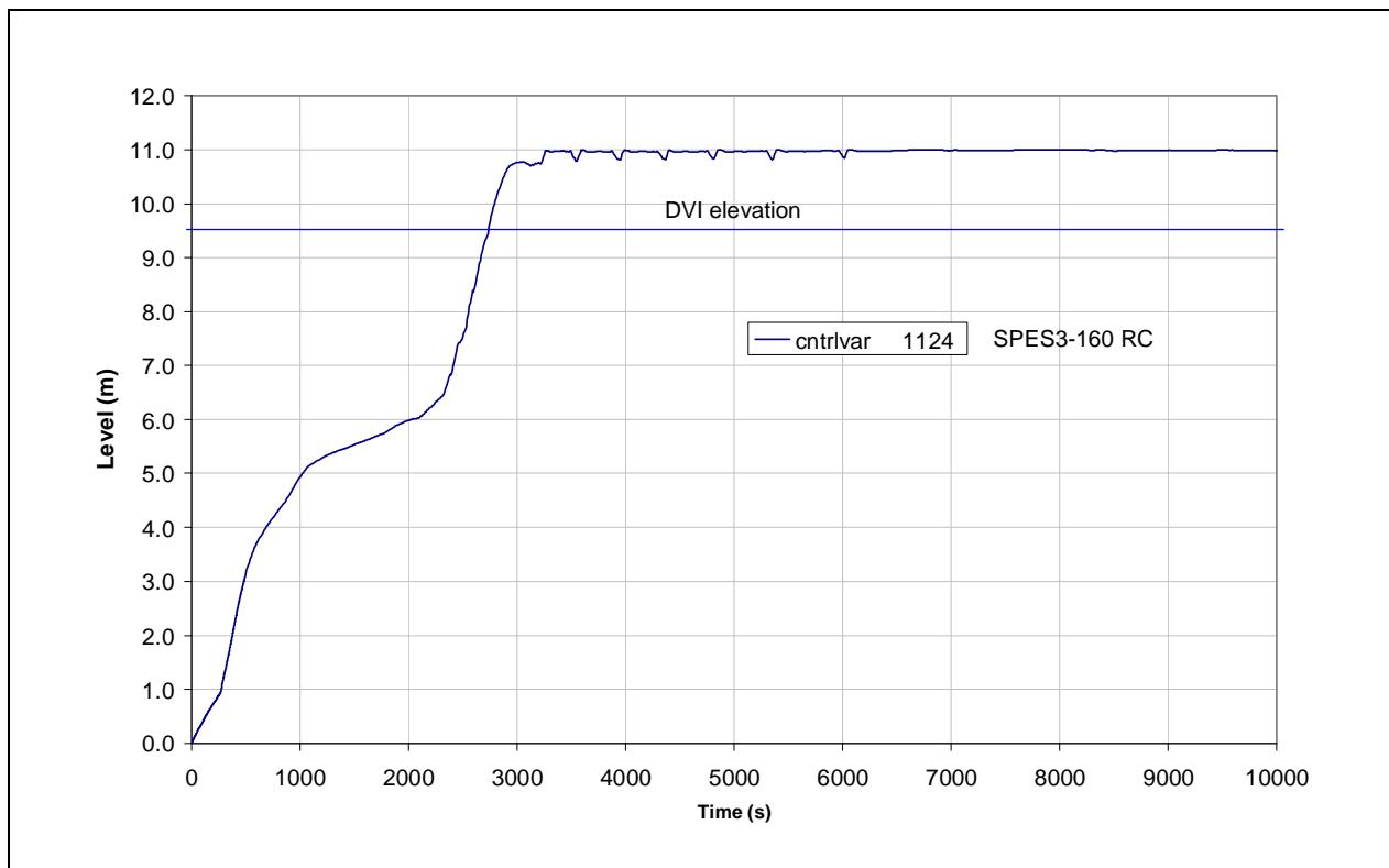
**Fig.4.30 – SPES3-160 RC level**
