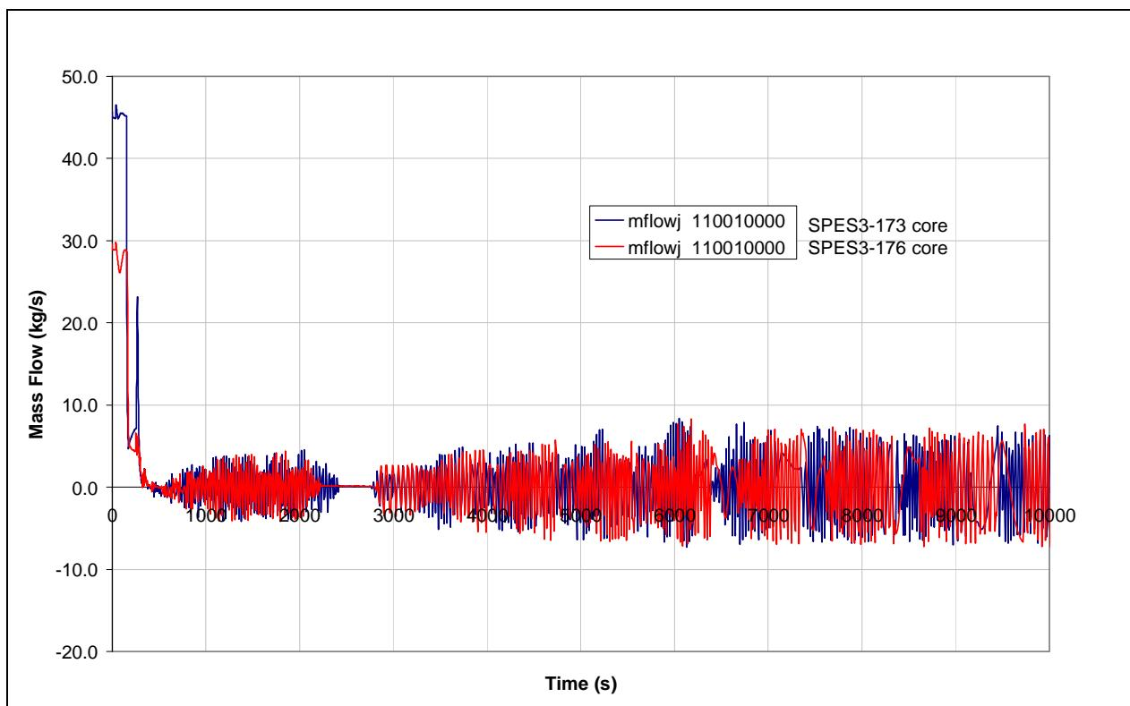
**Fig.8. 57 – SPES3-173 and SPES3-176 core inlet flow**
