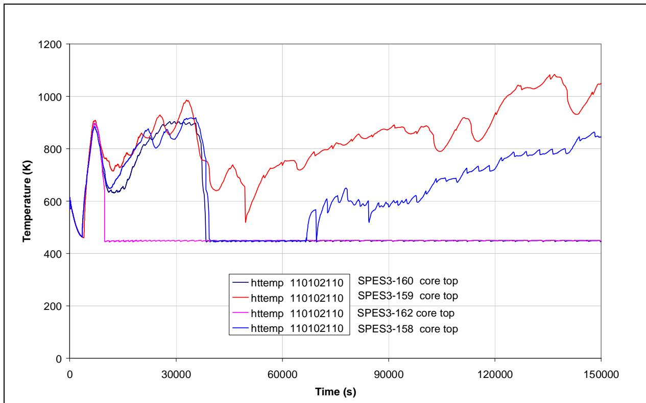
**Fig.5. 14 – SPES3-159, 162, 158 and 160 Core heater rod clad surface temperature (hot rods)**
