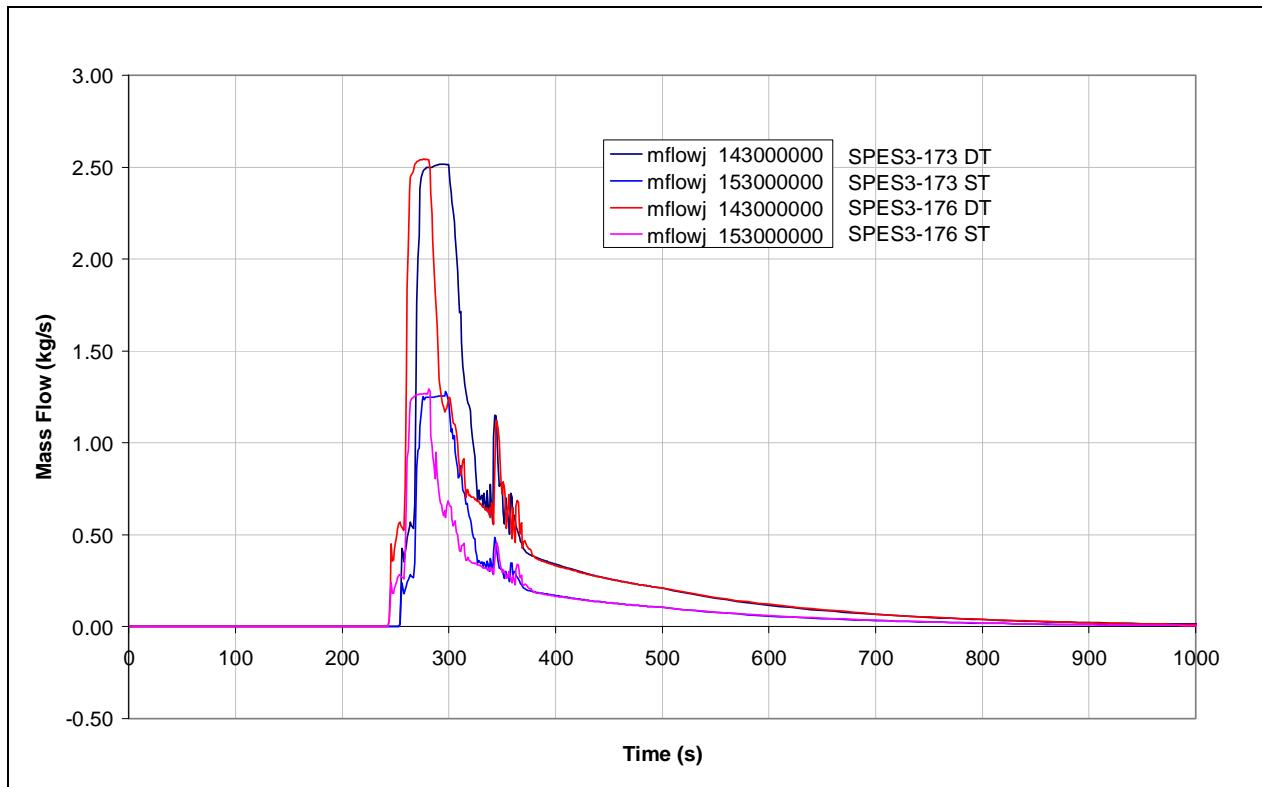
**Fig.8. 8 – SPES3-173 and SPES3-176 ADS Stage-I mass flow (window)**
