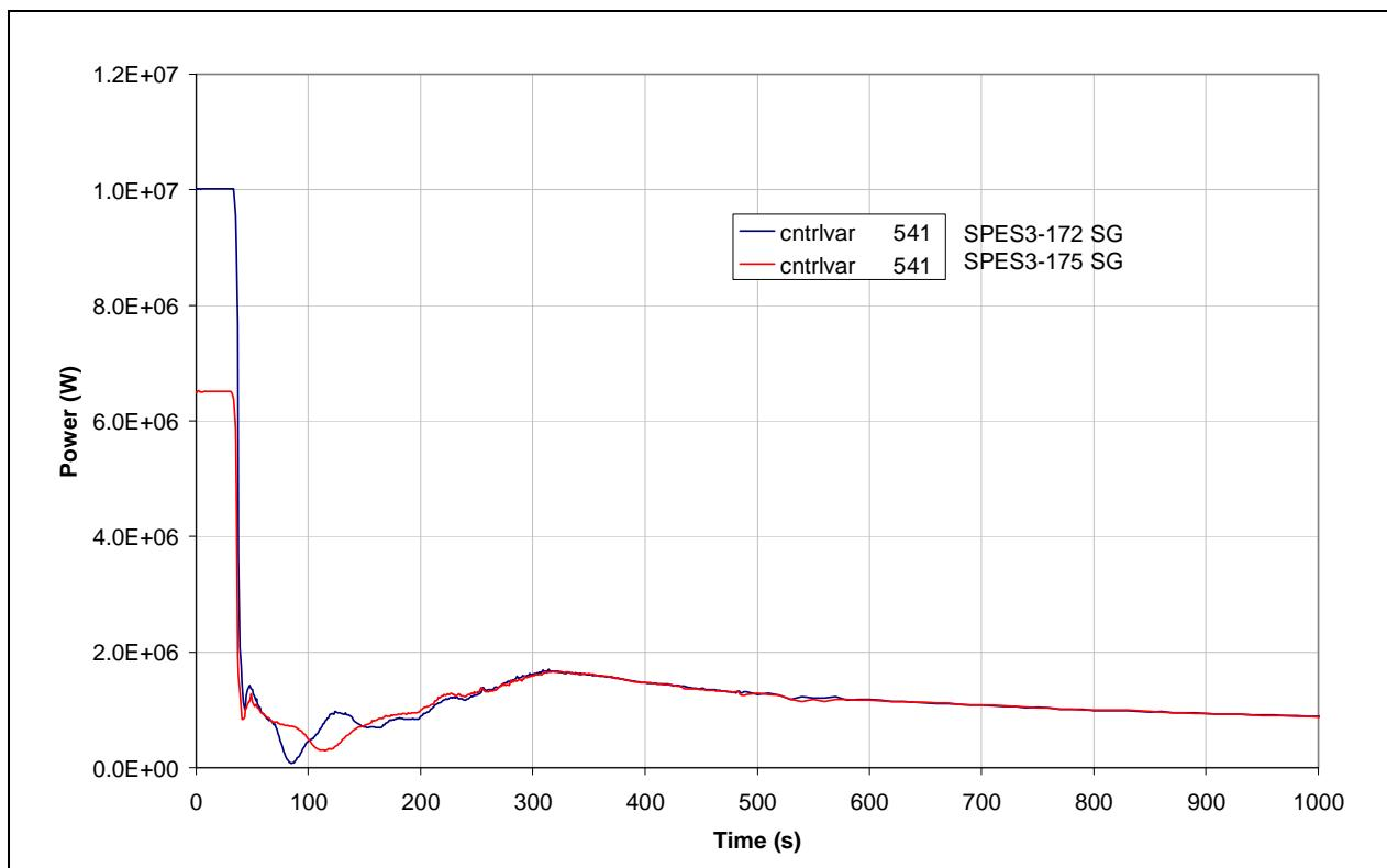
**Fig.7. 34 - SPES3-172 and SPES3-175 SG power**
