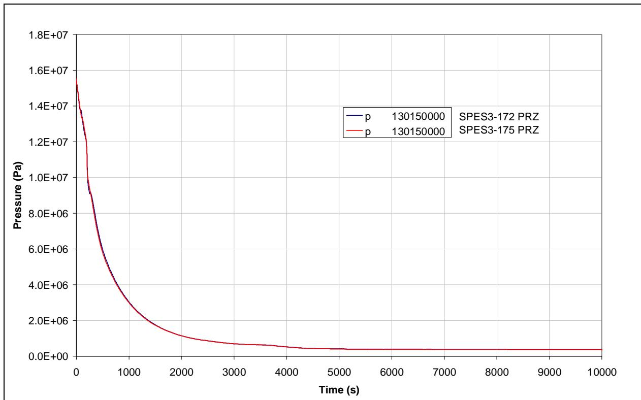
**Fig.7. 10 - SPES3-172 and SPES3-175 PRZ pressure**
