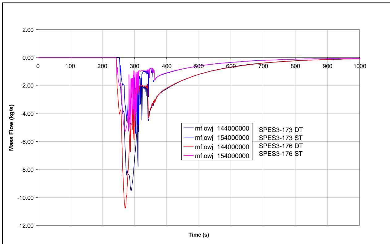
**Fig.8. 10 – SPES3-173 and SPES3-176 ADS Stage-II mass flow (window)**
