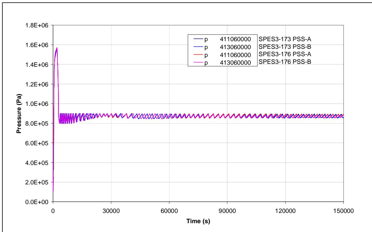
**Fig.8. 28 – SPES3-173 and SPES3-176 LGMS pressure (window)**
