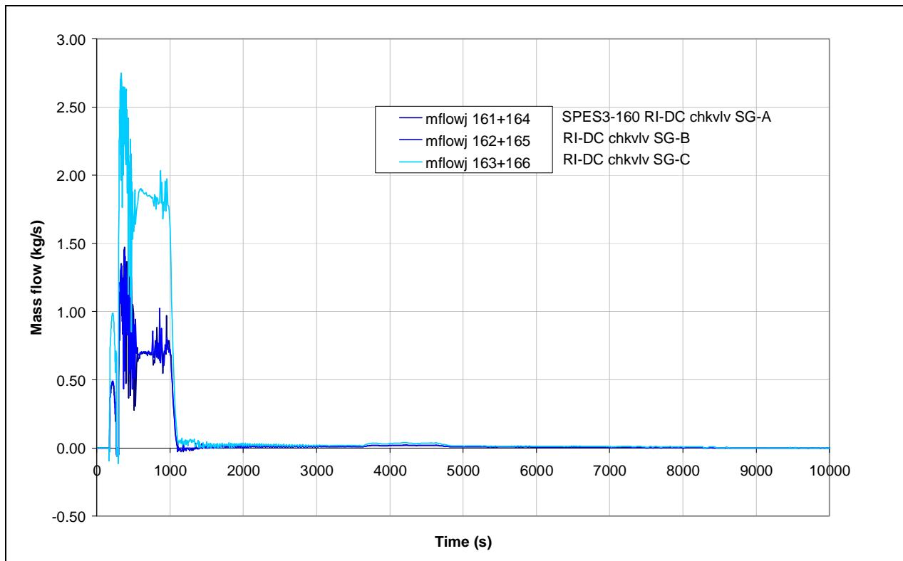
**Fig.4.50 – SPES3-160 RI-DC check valve mass flow**
