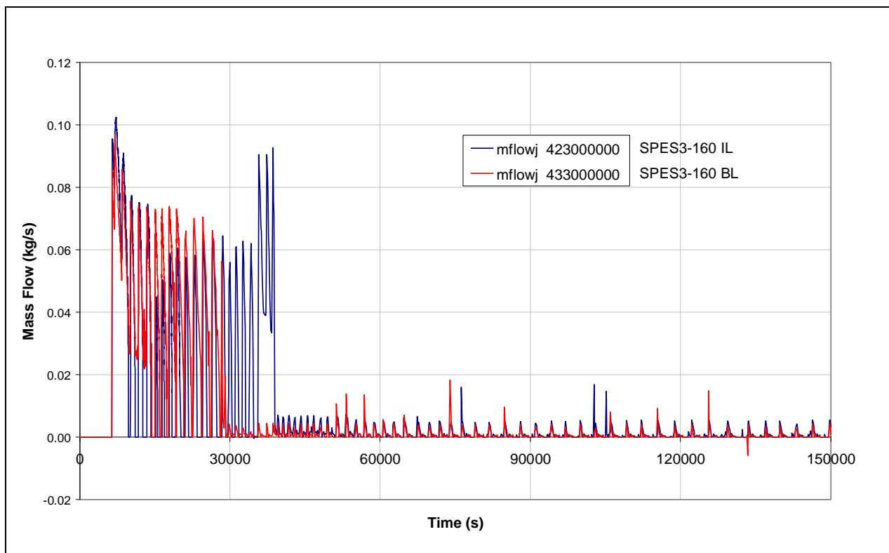
**Fig.4.5 – SPES3-160 ADS Stage-II mass flow**
