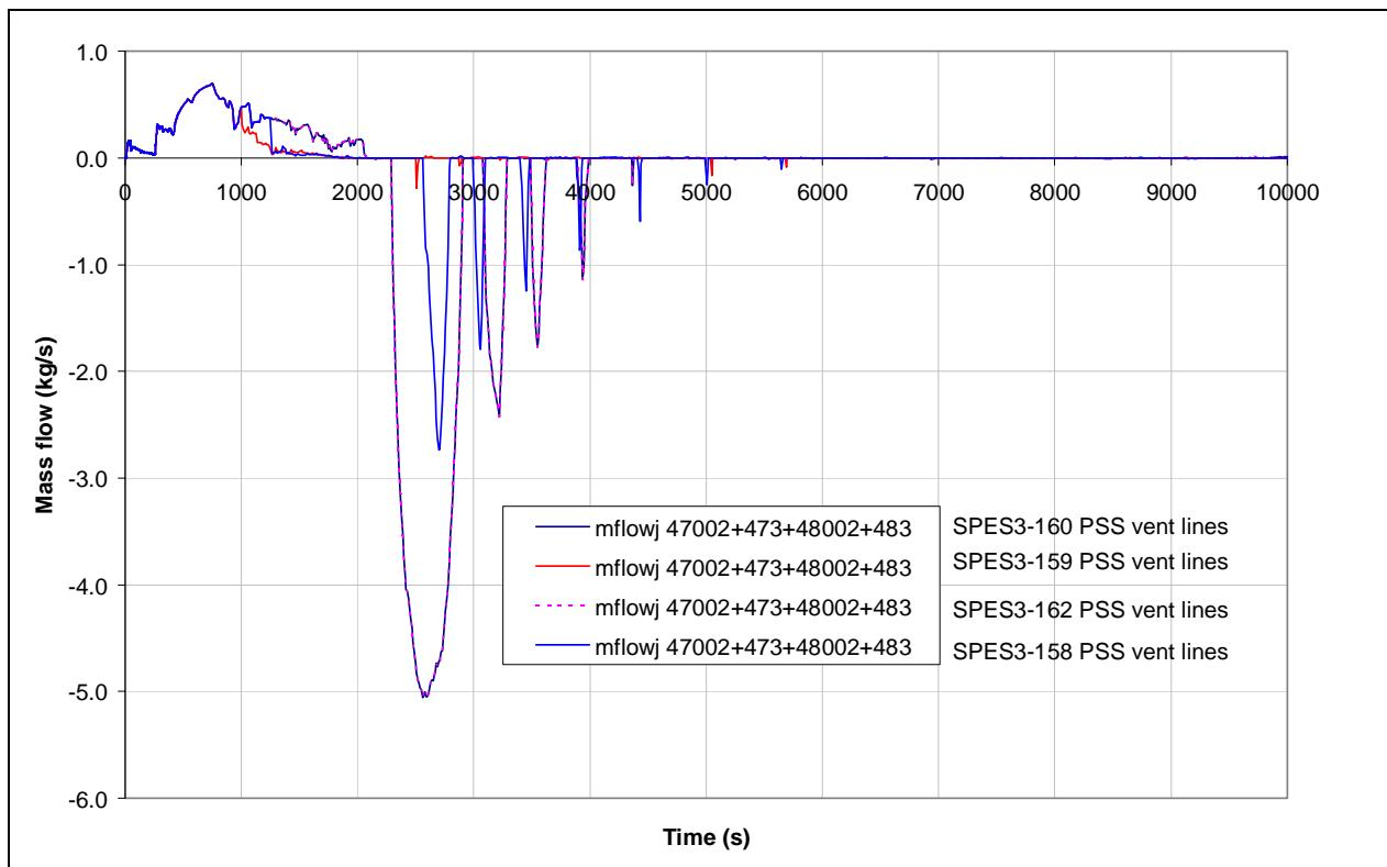
**Fig.5. 6 – SPES3-159, 162, 158 and 160 PSS to DW mass flow**
