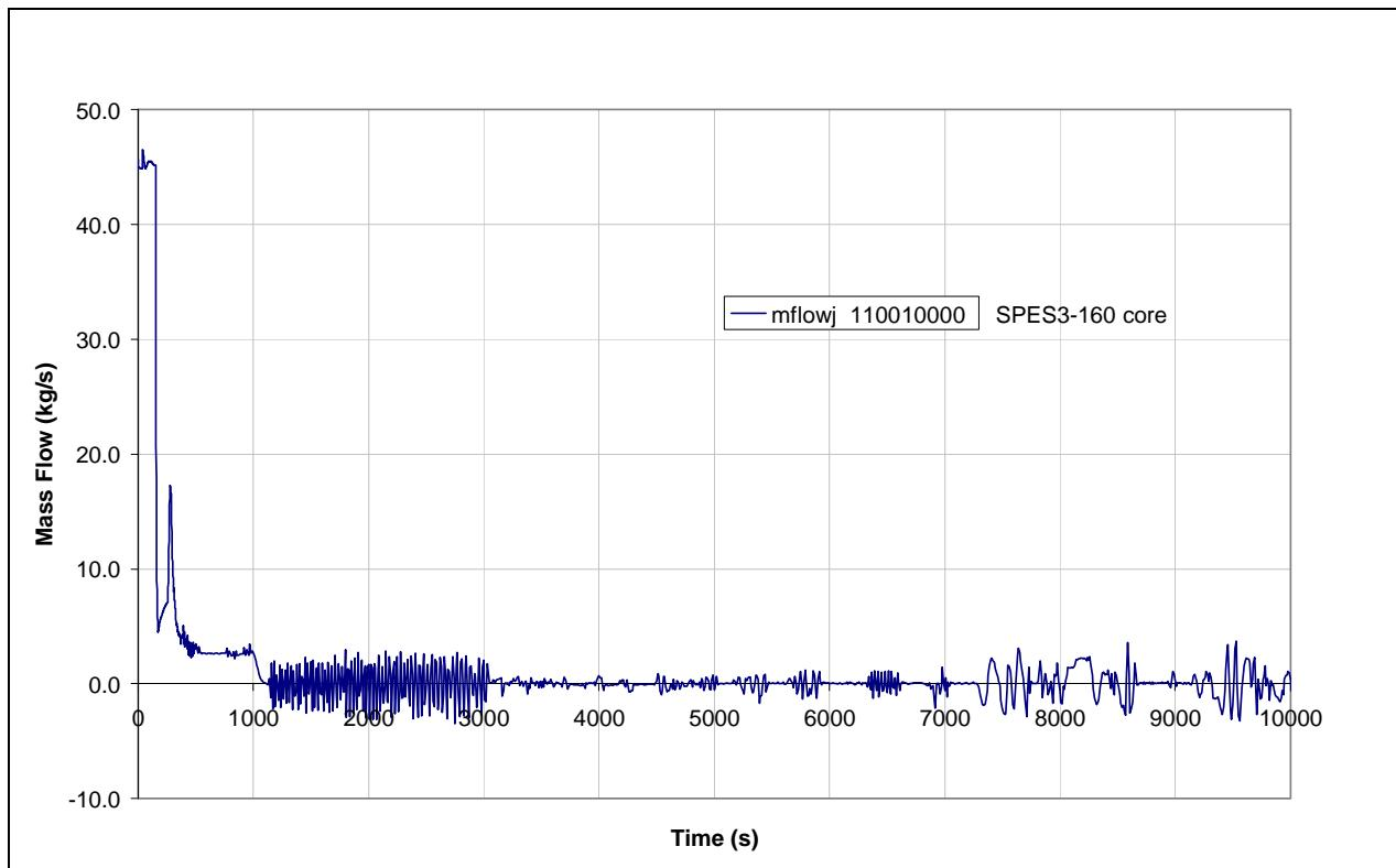
**Fig.4.48 – SPES3-160 core inlet flow**
