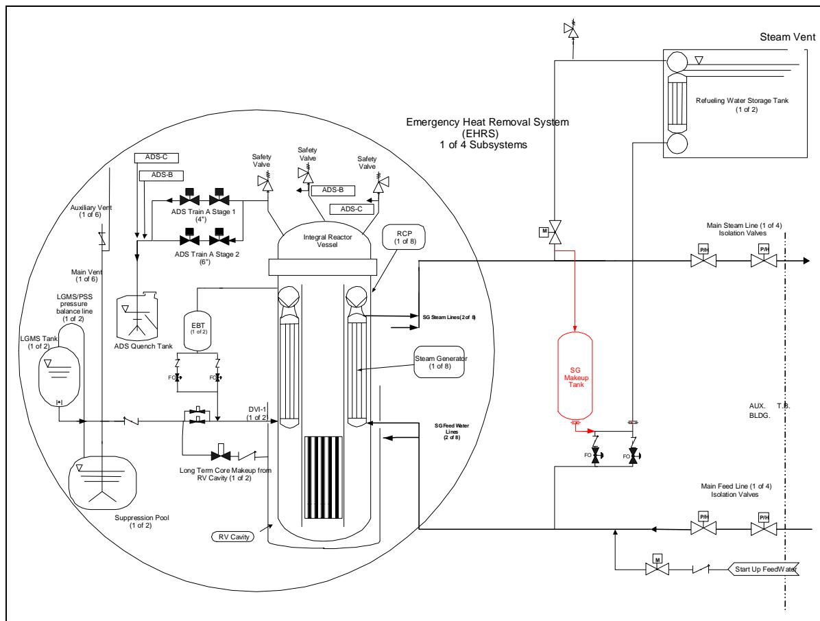
**Fig.3. 10 – IRIS Primary, Secondary and EHRS systems RELAP5 nodalization**
