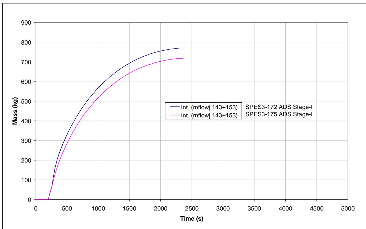
**Fig.7. 56 - SPES3-172 and SPES3-175 RC to DVI mass flow IL (window)**
