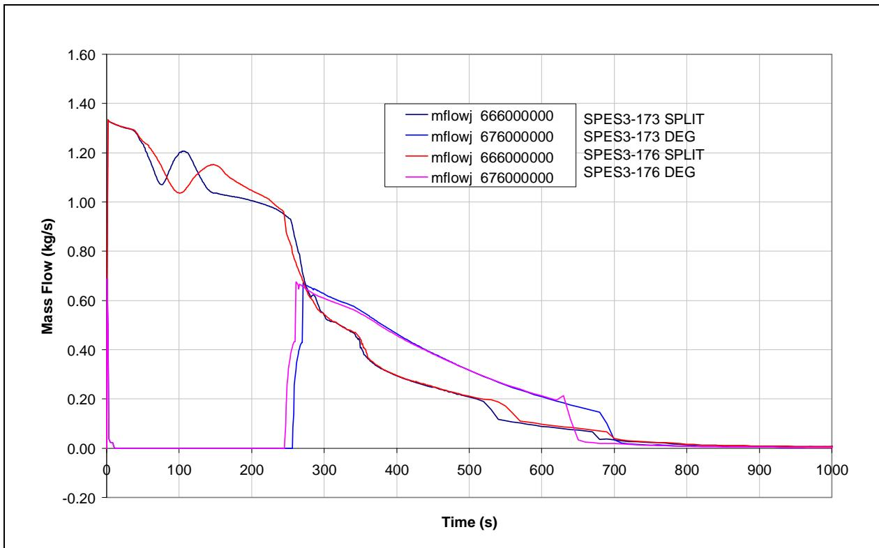
**Fig.8. 2 – SPES3-173 and SPES3-176 DVI line break flow (window)**
