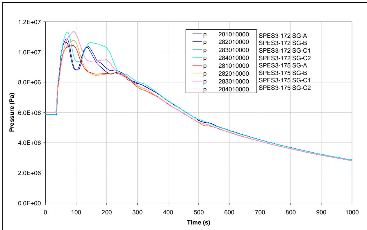
**Fig.7. 42 - SPES3-172 and SPES3-175 SG ss outlet pressure**
