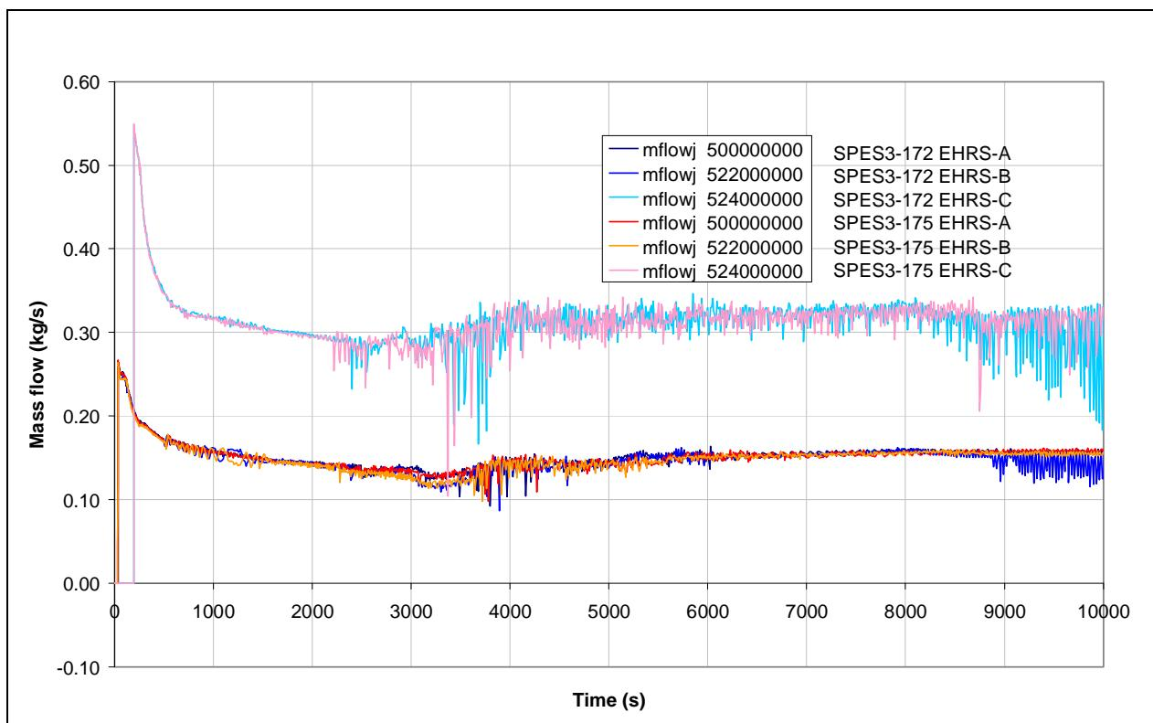
**Fig.7. 38 - SPES3-172 and SPES3-175 EHRS cold leg mass flow**
