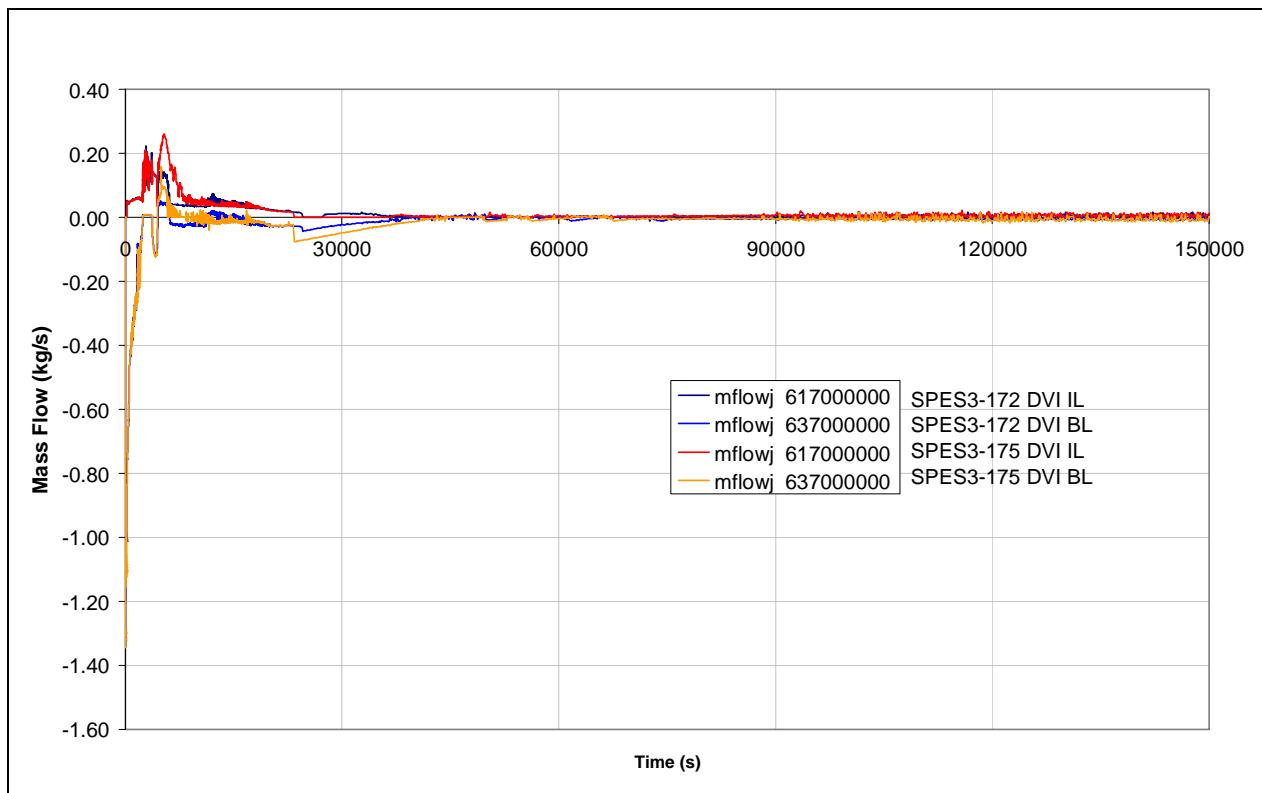
**Fig.7. 70 - SPES3-172 and SPES3-175 QT level**
