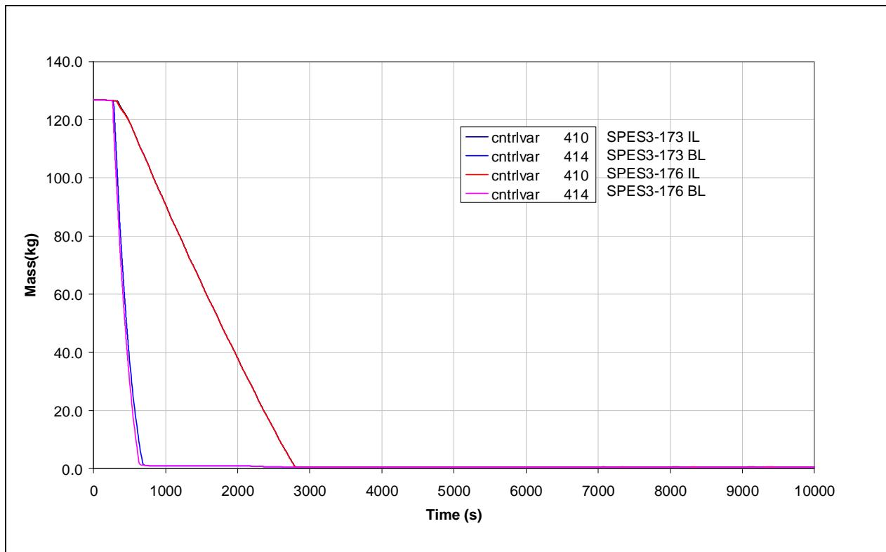
**Fig.8. 62 – SPES3-173 and SPES3-176 EBT level**
