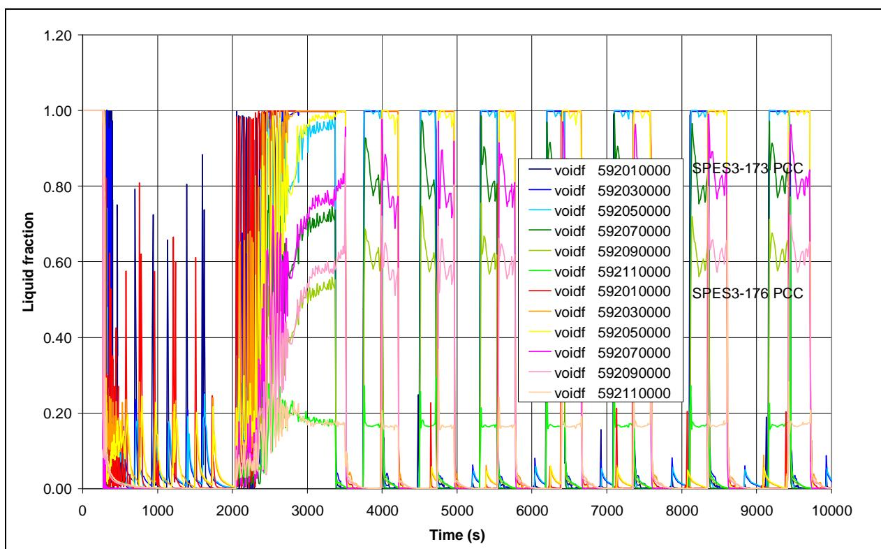
**Fig.8. 79 – SPES3-173 and SPES3-176 PCC liquid void fraction**
