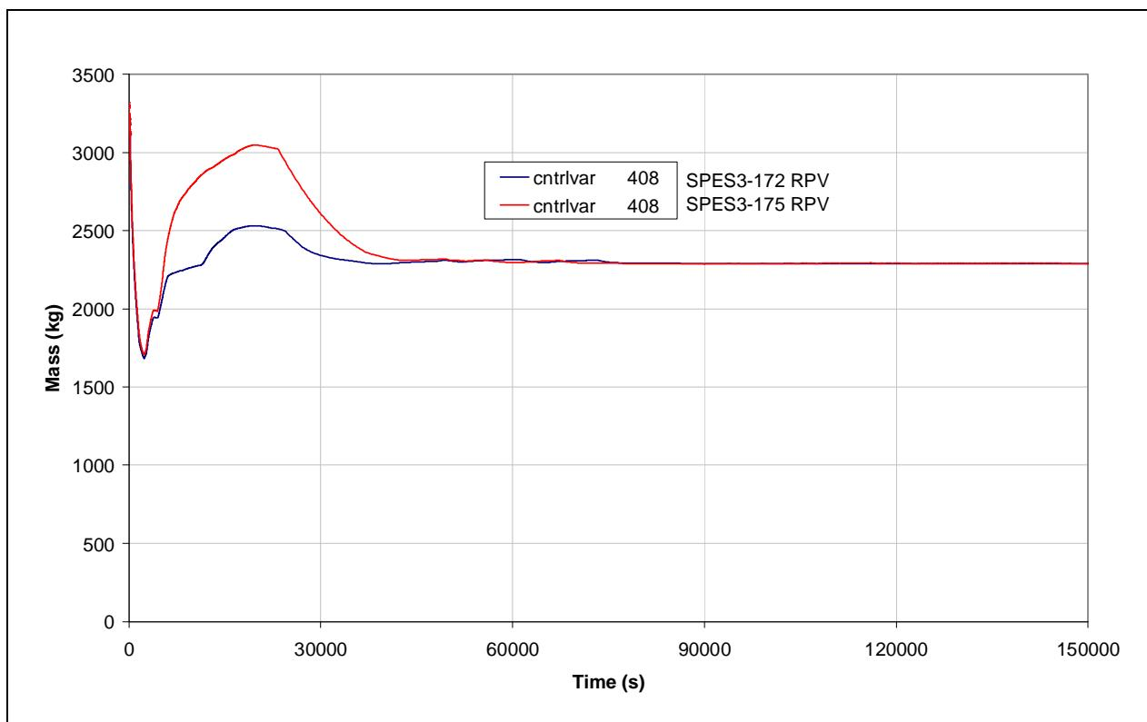
**Fig.7. 54 - SPES3-172 and SPES3-175 Core liquid fraction (window)**
