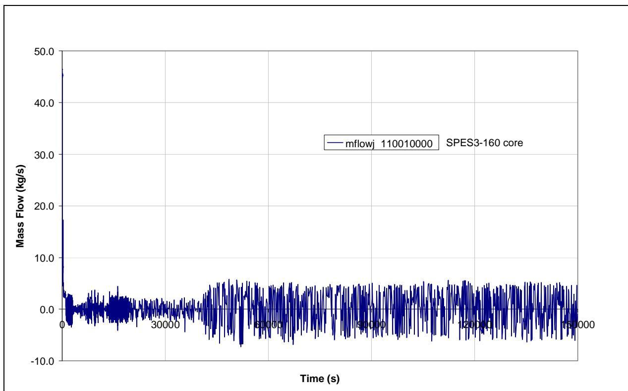
**Fig.4.49 – SPES3-160 RI-DC check valve mass flow (window)**
