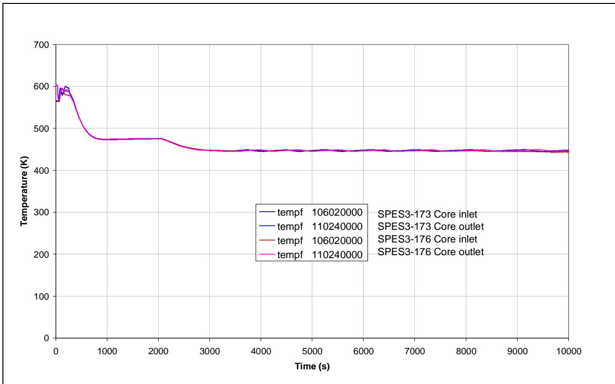
**Fig.8. 70 – SPES3-173 and SPES3-176 Core inlet and outlet temperatures**
