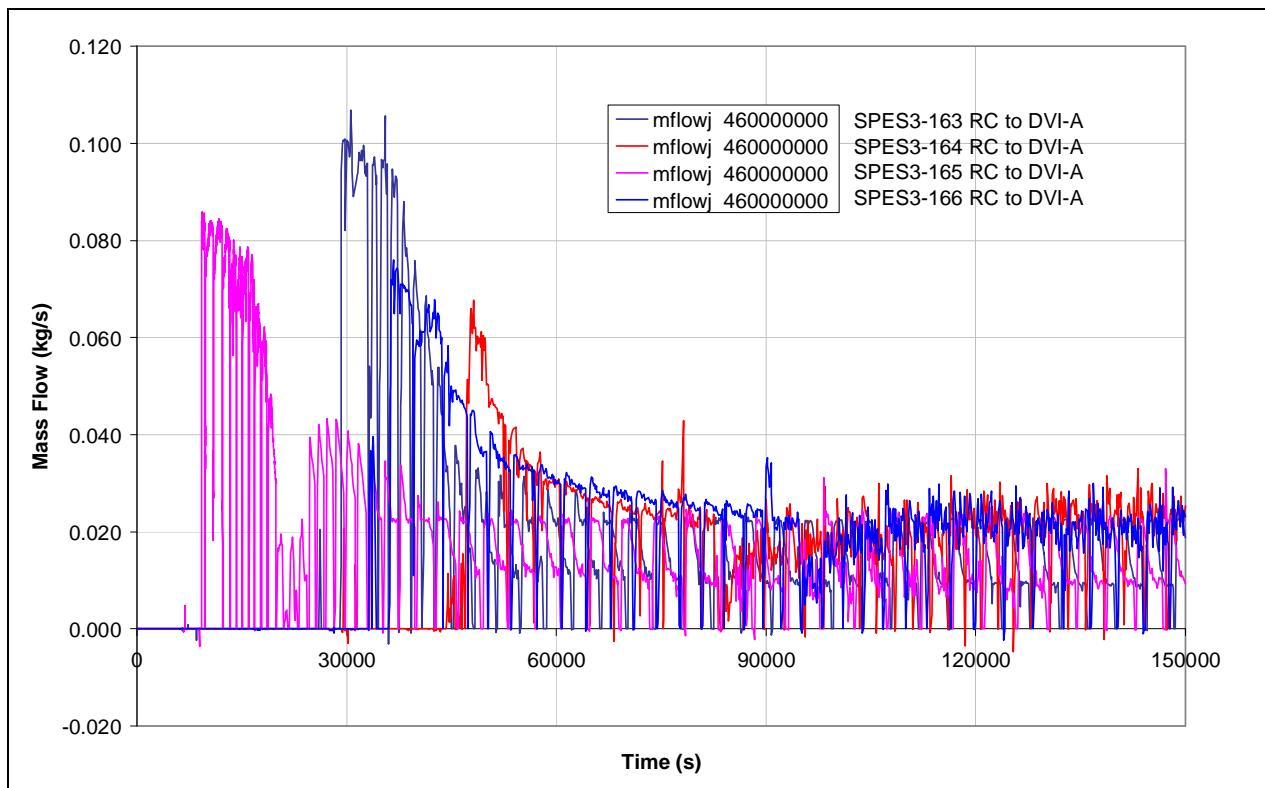
**Fig.5. 25 – SPES3-163, 164, 165 and 166 DVI break line (RPV side) mass flow (window)**
