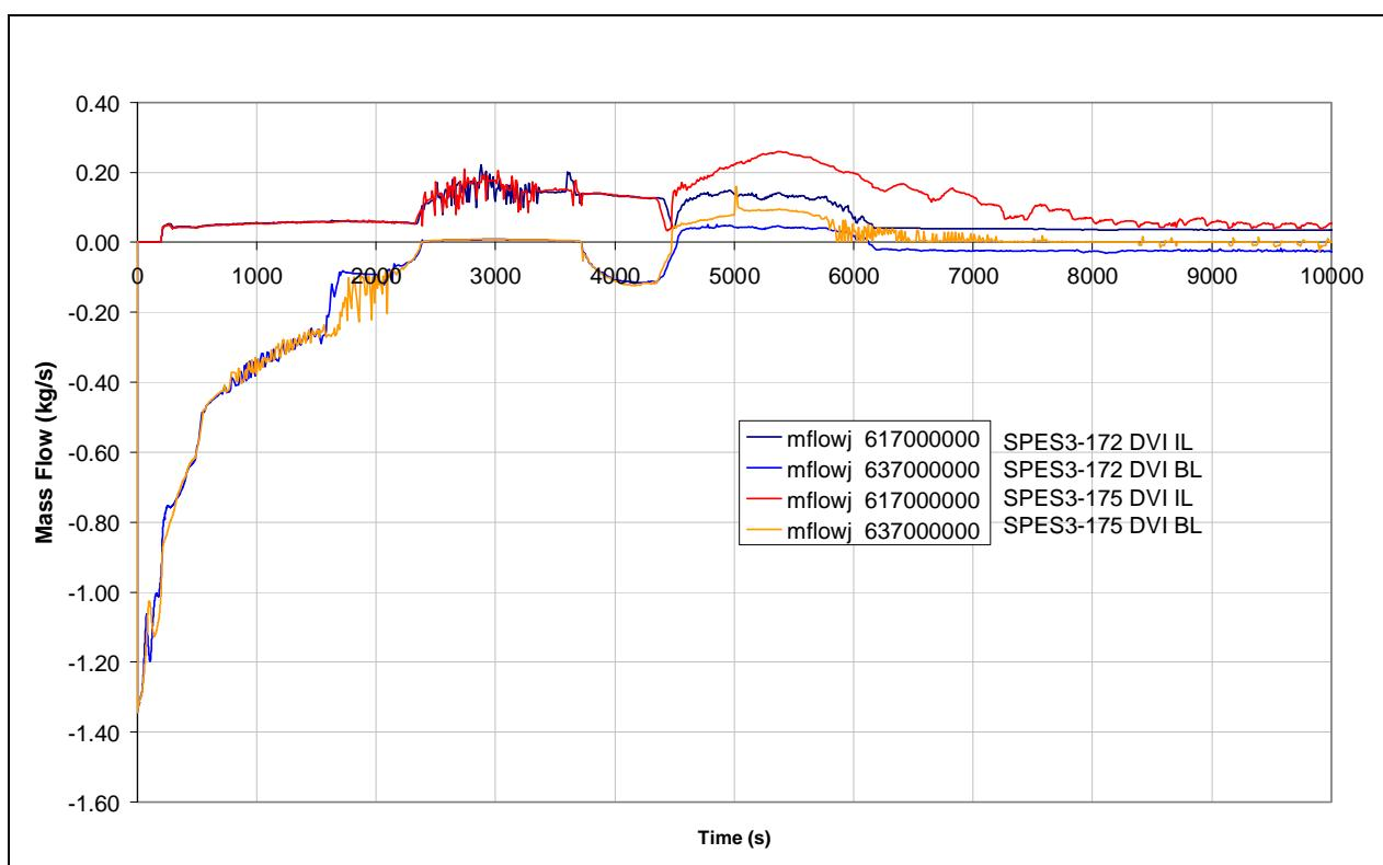
**Fig.7. 69 - SPES3-172 and SPES3-175 DVI mass flow**
