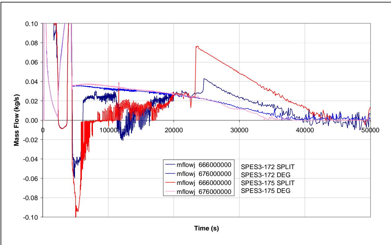
**Fig.7. 4 - SPES3-172 and SPES3-175 DVI break mass flow**
