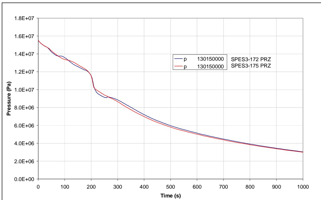
**Fig.7. 9 - SPES3-172 and SPES3-175 PRZ pressure (window)**
