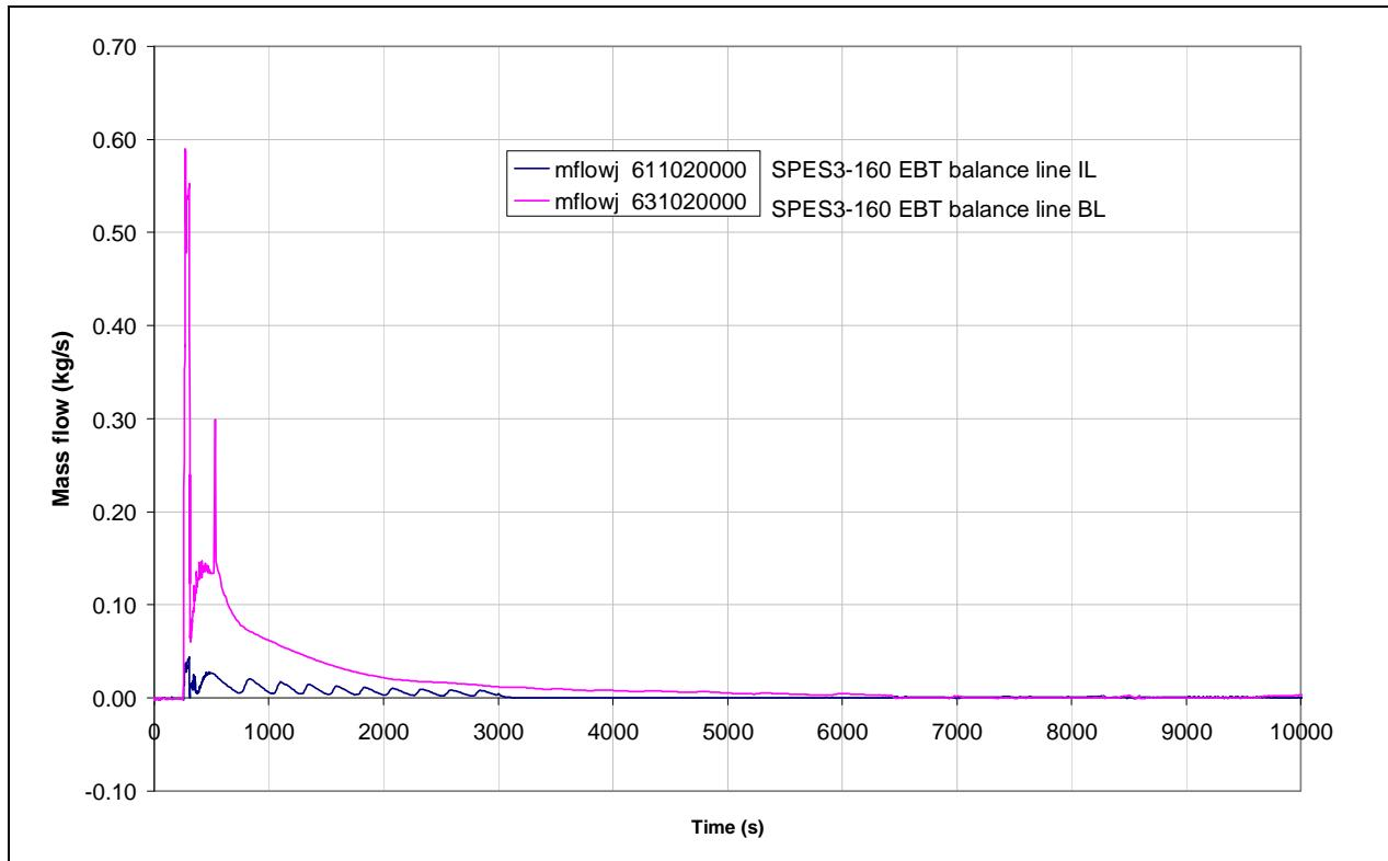
**Fig.4.54 – SPES3-160 EBT balance line mass flow**
