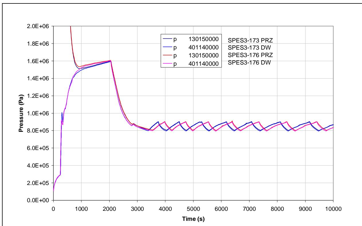
**Fig.8. 13 – SPES3-173 and SPES3-176 PRZ and DW pressures (window)**
