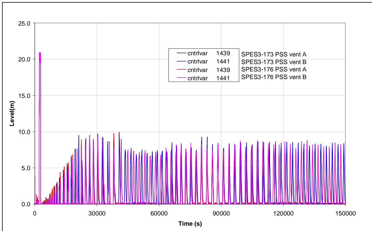
**Fig.8. 34 – SPES3-173 and SPES3-176 PSS level (window)**
