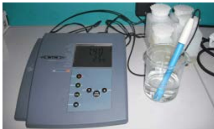
Figura 6.1. pH-metro (WTW- InoLab pH720).
