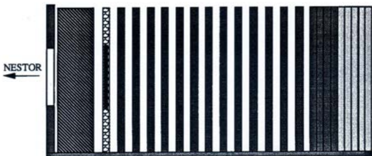
Figure 1 Schematic side elevation of the shield in the iron 88 single material benchmark experiment
