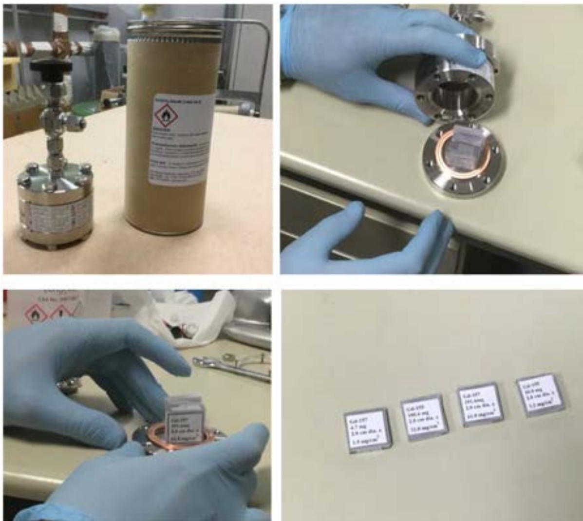
Fig. 4 Gadolinium-odd samples as shipped in an airtight underpressurized cask (upper left hand corner). On the bottom right one: the four Gd samples used for the experimental campaign.
