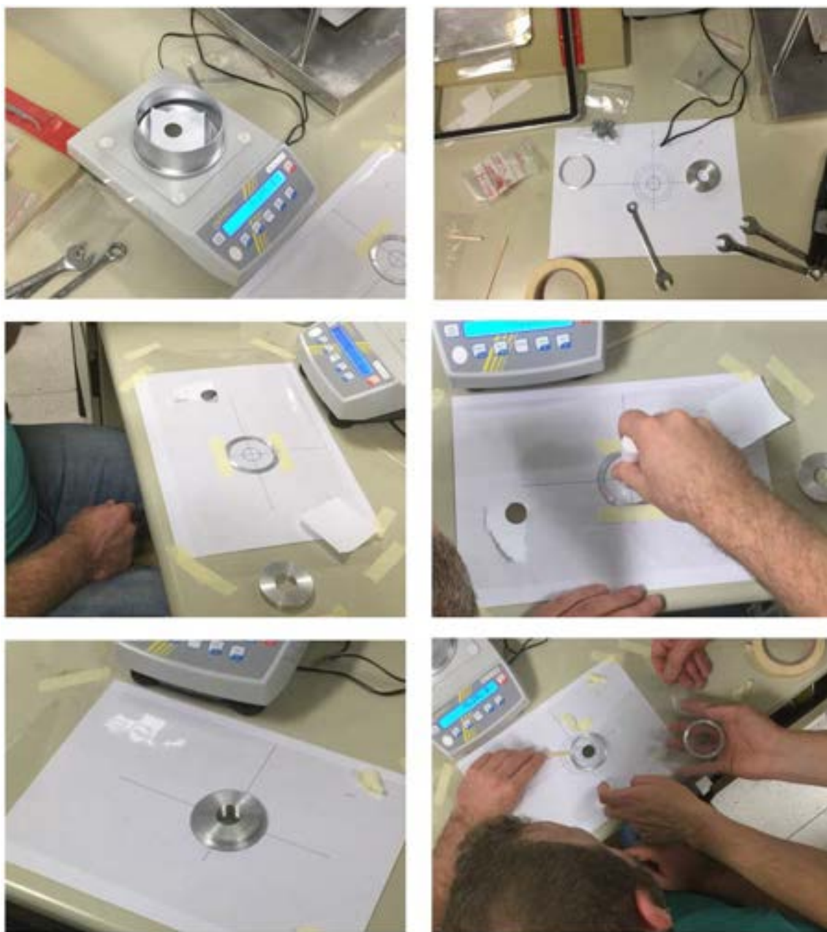
Fig. 5: Preparation of the samples for their arrangement in annular frames to get the correct positioning on the flight path during the experimental campaign.
