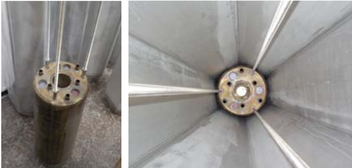
Figure 5.2 View of the ALFRED test section (left) and its positioning in the central hexagonal channel (right).
