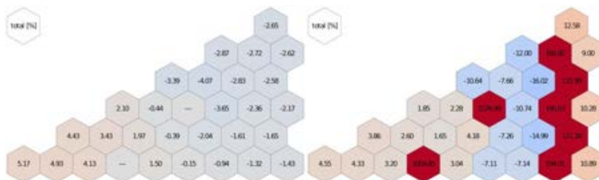
Figure 17. Relative variation of the shape of the deposited power with respect to the initial distribution after 10 s: without photon transport (Scenario 1 and Scenario 2, left) and with photon transport (Scenario 3, right); see Table 4.
