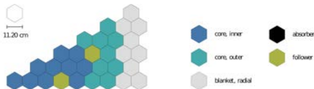
Figure 14. Configuration of the system analysed. The transient is initiated by instantaneously replacing the «follower» material by the «absorber» material.
