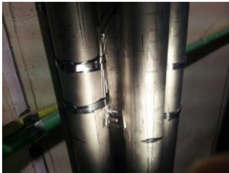
Fig. 27 – Thermocouples in the lead sub-channel
