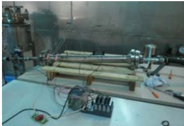
Figure 7 Flow meter and test rig used for the experimental tests in water.
