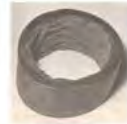
Slag in pipeline
