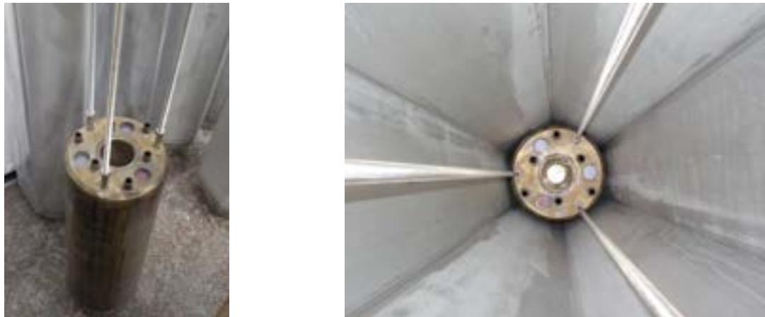
Figure 2.3 View of the ALFRED test section (left) and its positioning in the central hexagonal channel (right).
