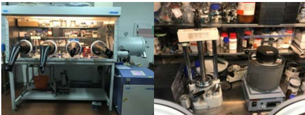
Fig. 6.3 – Manual press and furnace inside the glove box operating under inert atmosphere.
