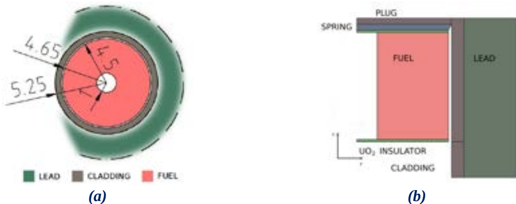
Fig. 8.4 – (a) Analysed fuel pin and surrounding lead. Radial sizes at nominal conditions (room temperature), expressed in mm. (b) Longitudinal (r; z) view of the modelled geometry.
