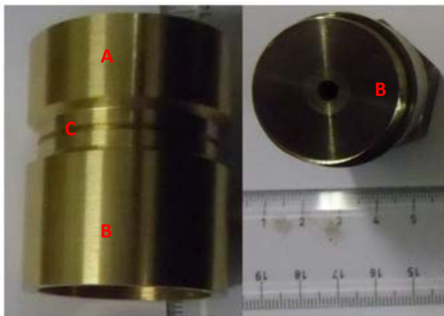
Fig. 9.5 – View of the protective cap “A” and injection orifice “B” (from [9.4]).
