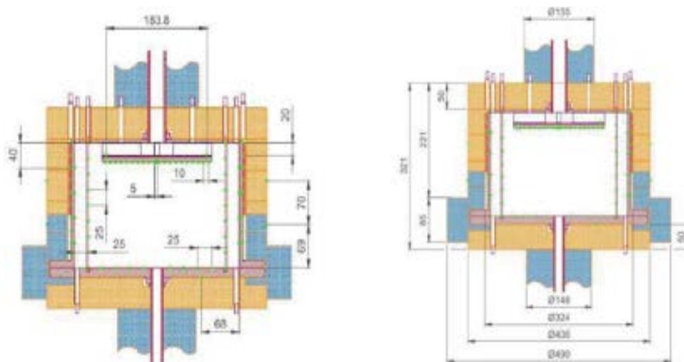
Fig. 4.8 - Modelling for TALL-3D. Geometry and dimensions.
