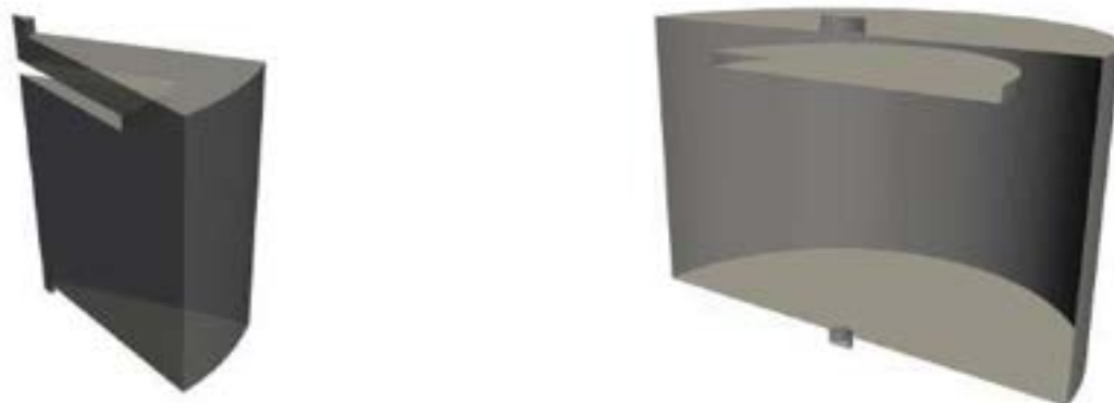
Fig. 4.11 - TrioCFD modelling for TALL-3D. Geometry of the axial-symmetric and three-dimensional test section.
