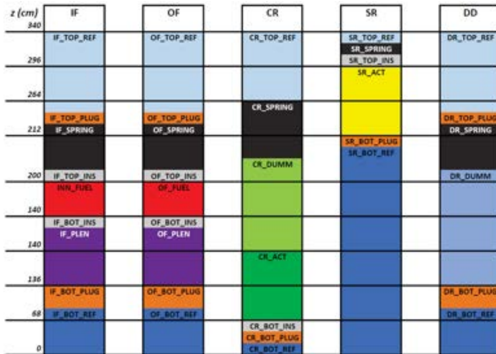
Fig. 5.15 – Axial discretization for the FRENETIC model (black lines) on top of fine Serpent axial discretization for each radial region.
