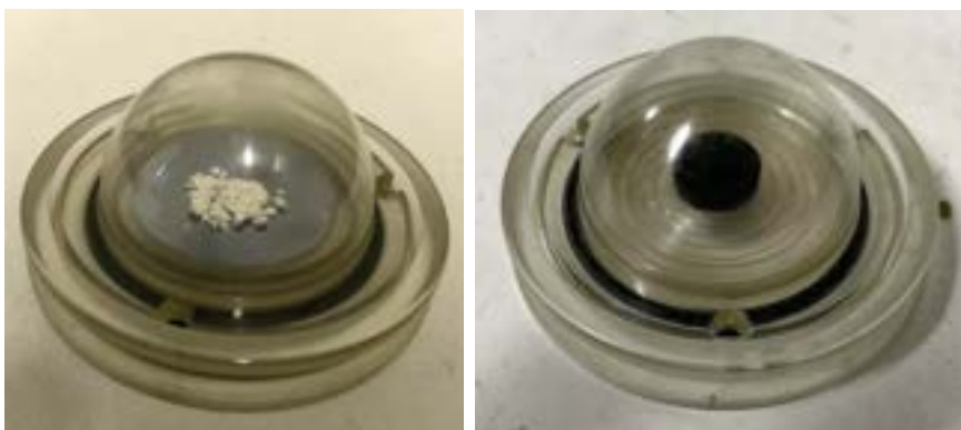
Fig. 8.5 – Sample holder for XRD analysis: \text{CeO}_2 (left) and \text{Fe}_2\text{O}_3 (right).
