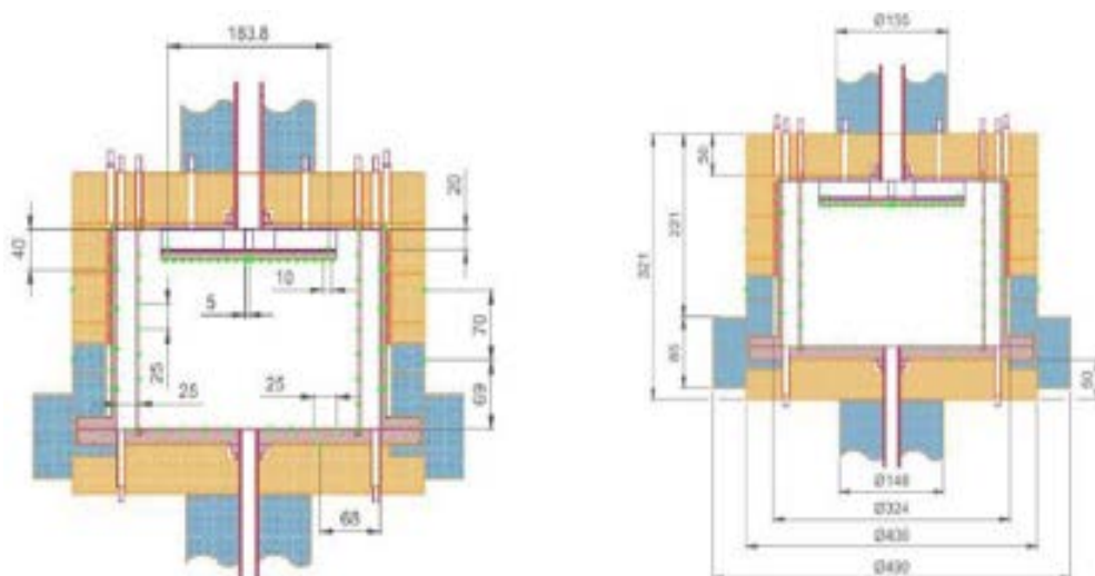
Fig. 4.5 - Modelling for TALL-3D. Geometry and dimensions.
