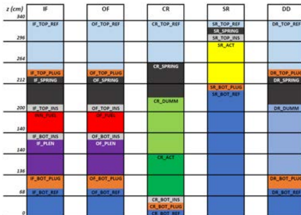
Fig. 5.5: ALFRED core configuration as in the benchmark calculations against Serpent/OpenFoam [5.1].
