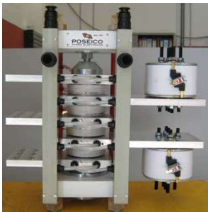
Figura 8 – Vista posteriore del CS1 power assembly.
