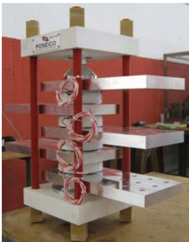
Figura 9 – Crowbar power assembly CS1/CS4
