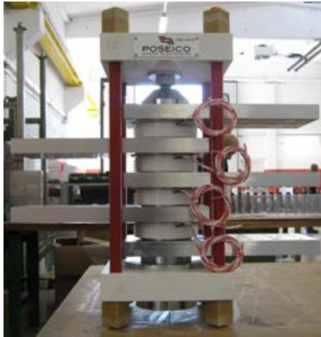
Figura 10- Crowbar power assembly CS1/CS4
