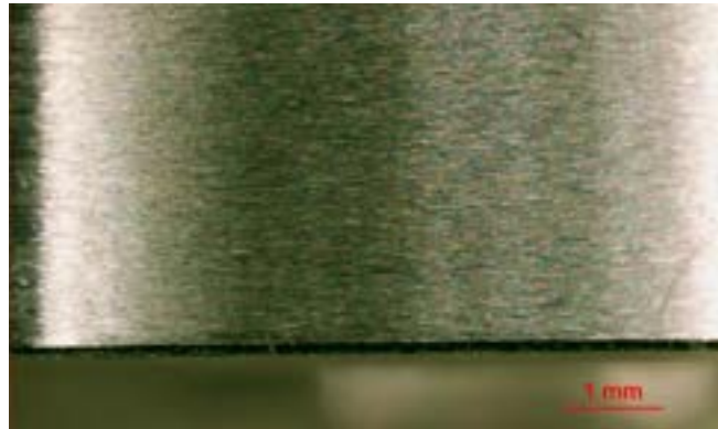
Figure 7: stereoscope image of a representative F82H specimen: curved external surface, viewed from the top. The surface is in good shape.
