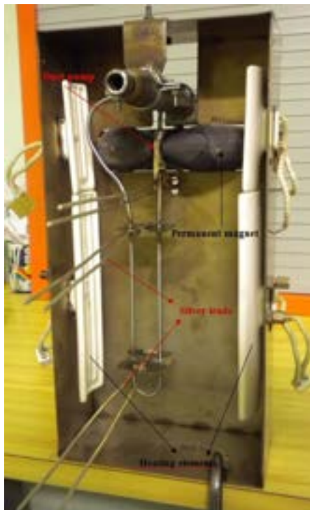
Figure 3: Real shot of the Resistivity Meter (prior of its installation inside Lifus 6 plant)
