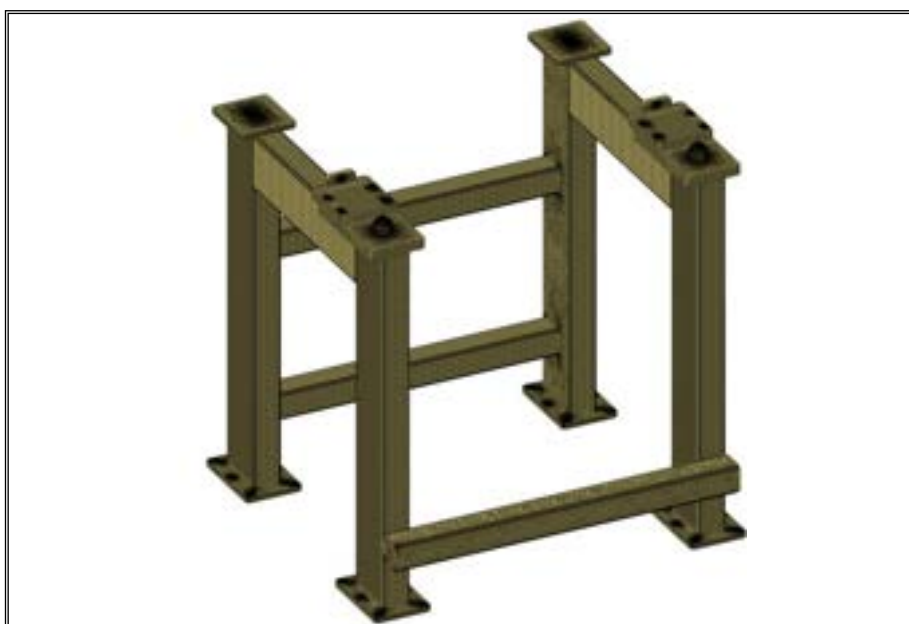
Figure 13. FEM model. Particular of the support framework.
