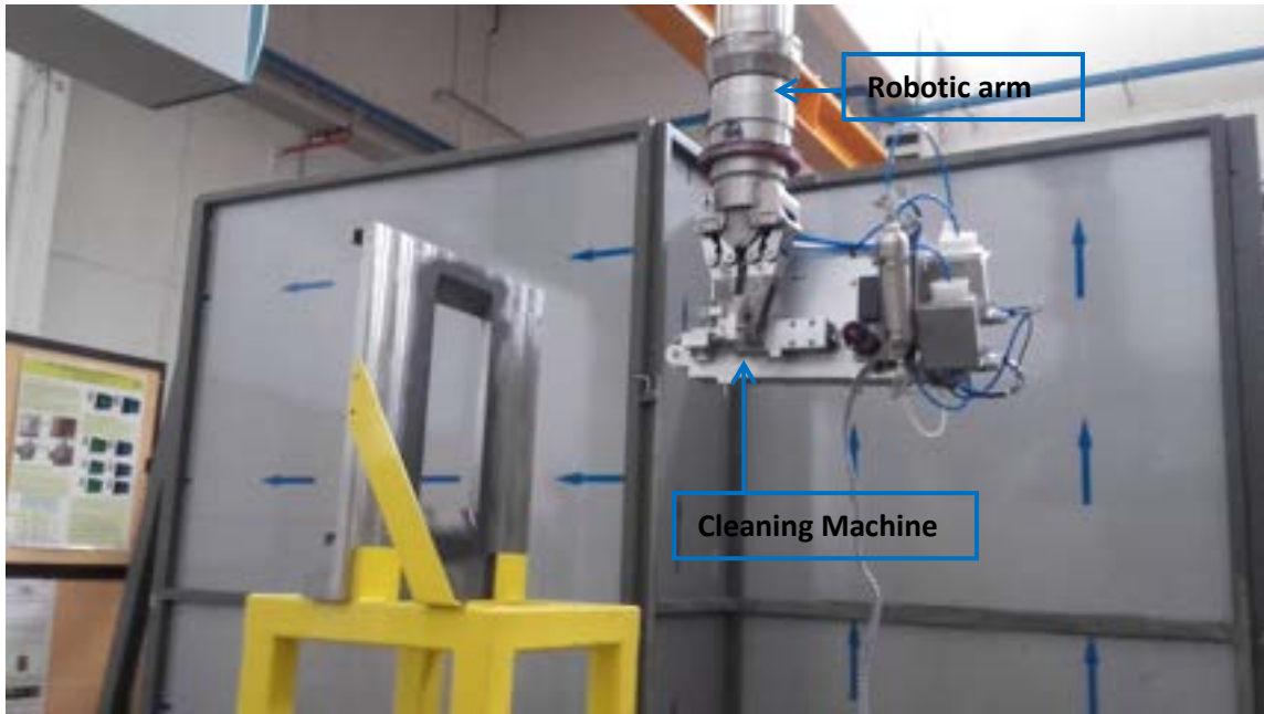
Fig. 17 Starting of cleaning operation
