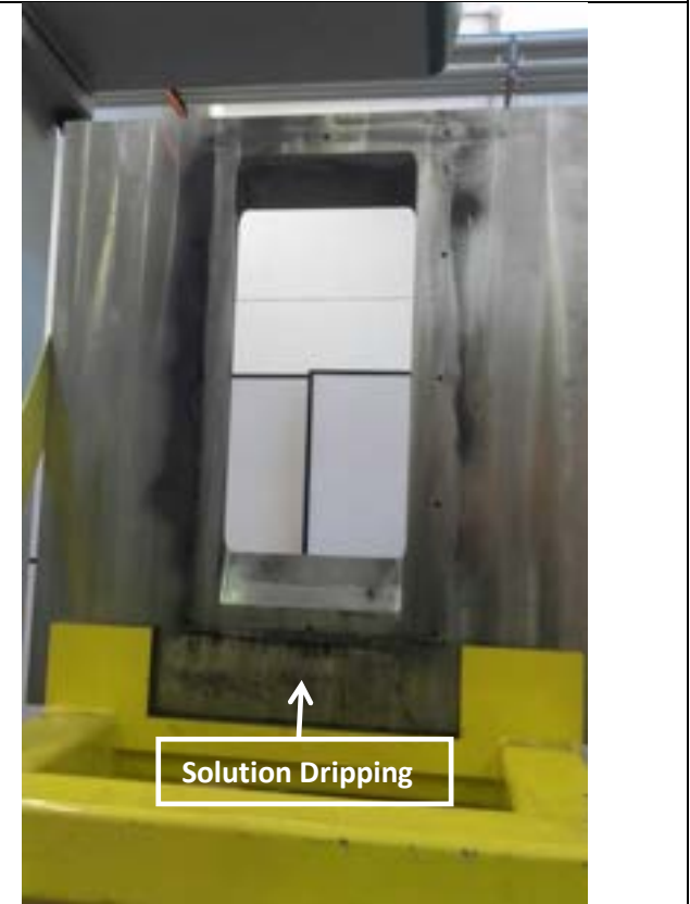
Fig.23 End cleaning phase
