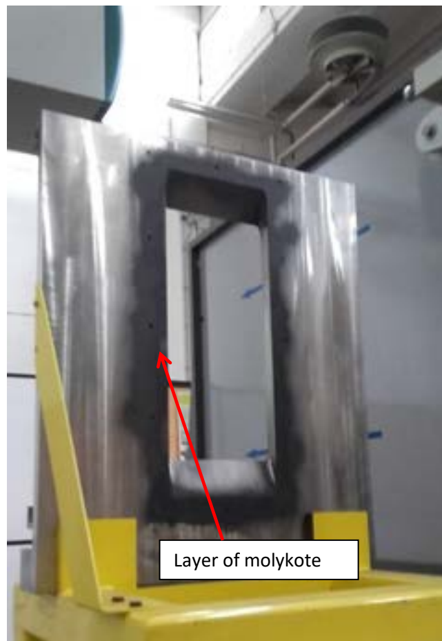
Fig. 16. Backplate support frame mockup sprayed with molykote
