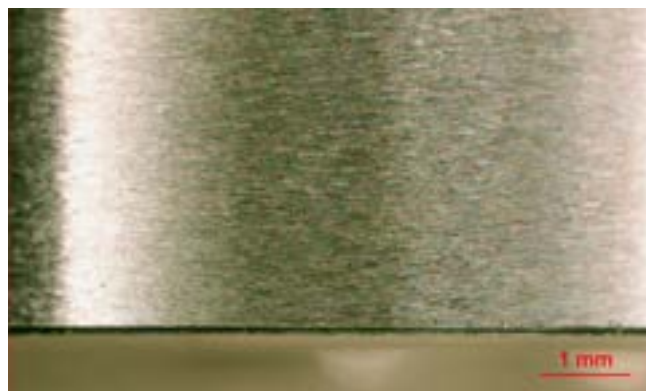
Figure 4: stereoscope image of a representative Eurofer 97 specimen: curved external surface, viewed from the top. The surface is in good shape.
