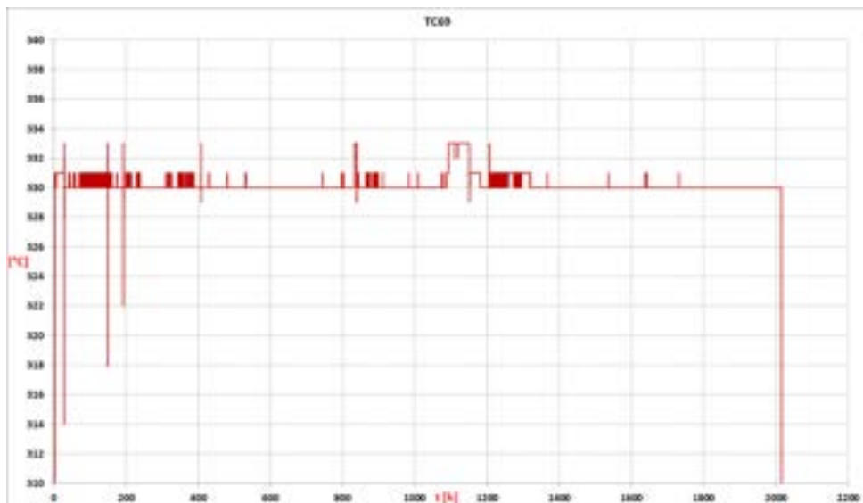
Figure 11: trend of the registered temperature of Lithium in the Test Section during the whole experimental test
