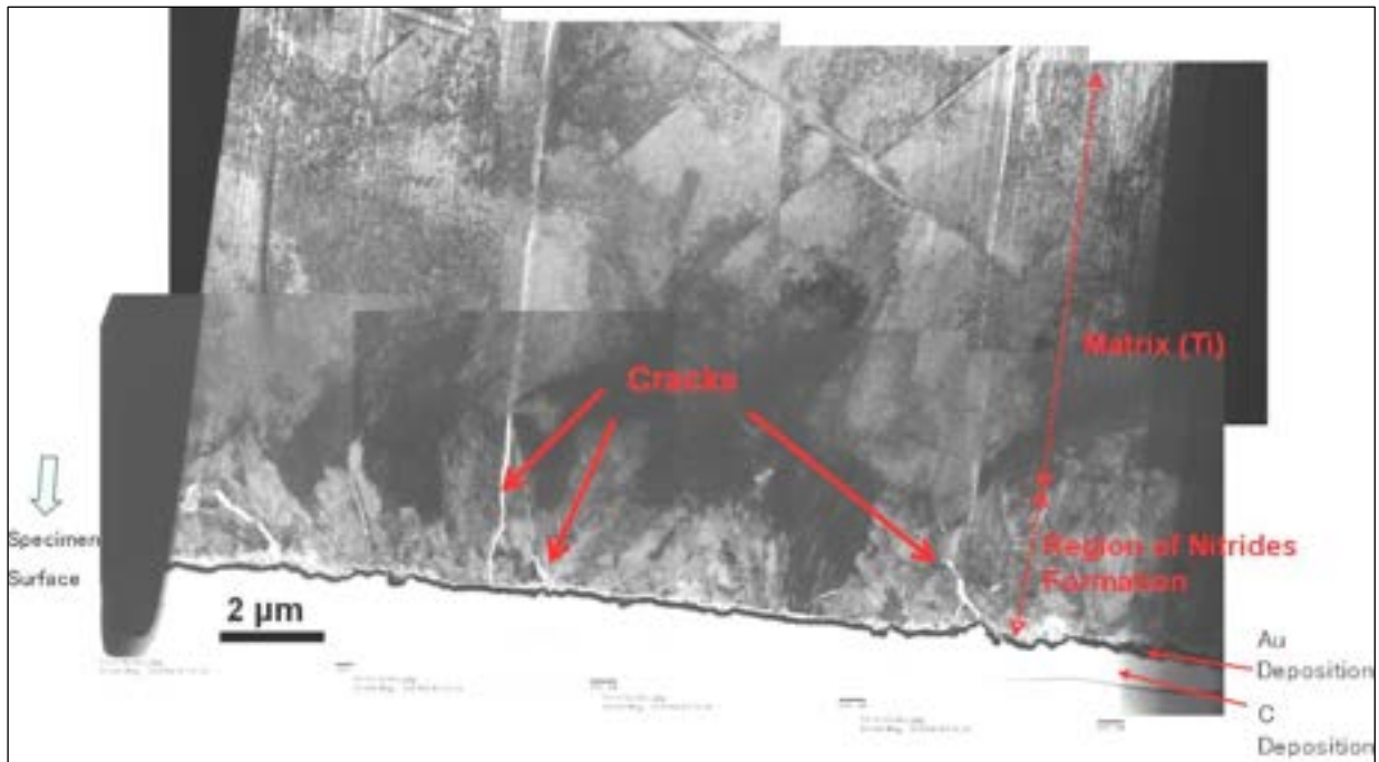
Figure 3: TEM image (Focused Ion Beam) of the Ti thin foil cross section after 27 h immersion at 600°C.
