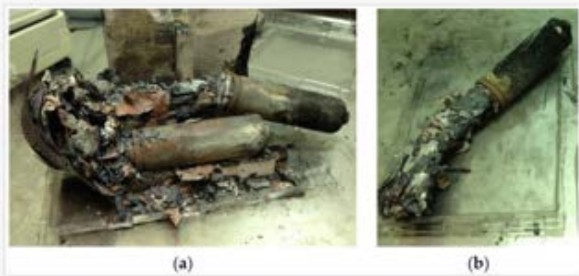
Figure 9. Photos of the exploded Lifetech cell during tear-down: (a) the exploded cell and part of the protection box and two adjacent cells; and (b) exploded cell alone.
