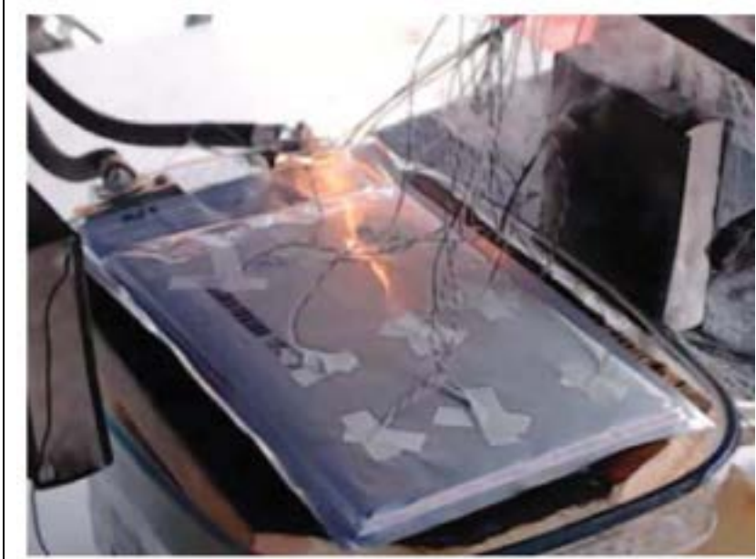
Figura 39. Short circuit for EiG batteries (new and old model) and for EB cell
