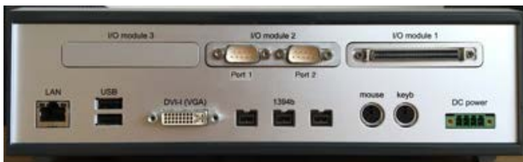
Figura 78: I/O di Speedgoat real-time target machine
