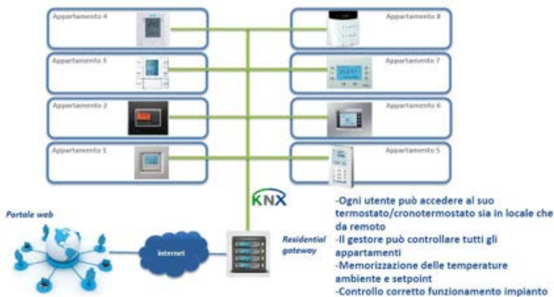
Figura 118. KNX web residential service gateway
