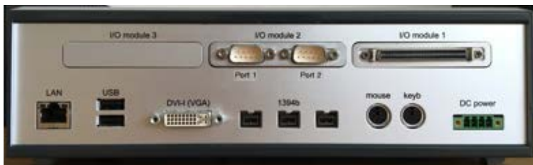
Figura 128: I/O di Speedgoat real-time target machine
