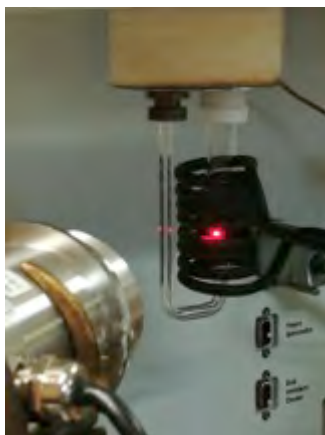
Figure 6. Inductor coil (d= 2.5cm, h=4.5cm) surrounding the reactor tube. A pyrometer provides an estimation of the catalyst surface temperature.
