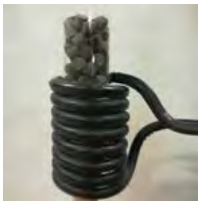
Figure 1: Example of a catalytic bed inside an induction coil. The catalyst material gets out of coil only for demonstration purposes.
