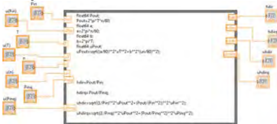
Fig 80 – Sub VI “rend dir temp inc”: block diagram
