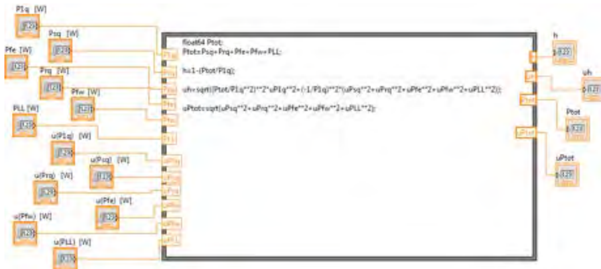
Fig 76 – Sub VI “rend indir inc”: block diagram
