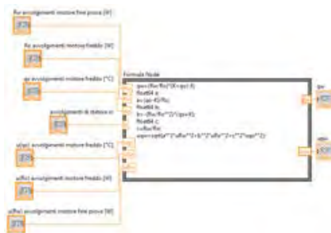
Fig 14 – Sub VI “temp stat avv inc”: block diagram
