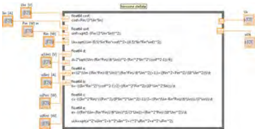
Fig 42 – Sub VI “tens int p fer inc”: block diagram
