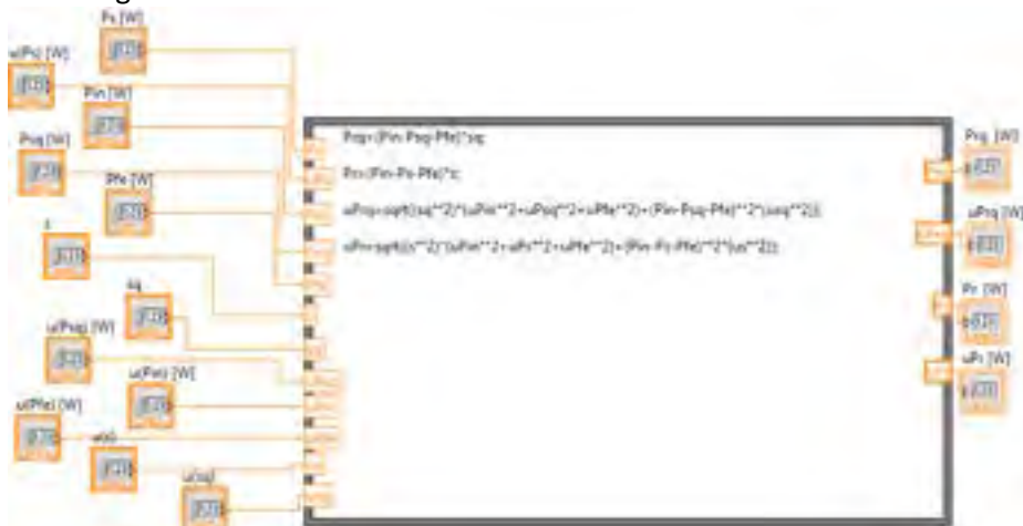
Fig 54 – Sub VI “perd rot corr inc”: block diagram
