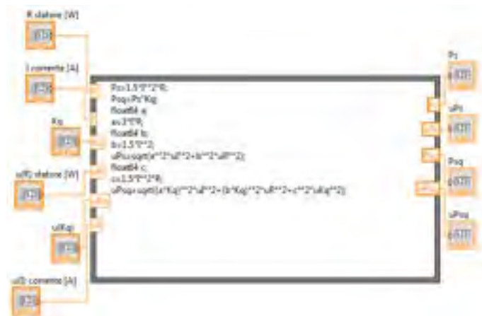
Fig 26 – Sub VI “perd avv stat inc”: block diagram
