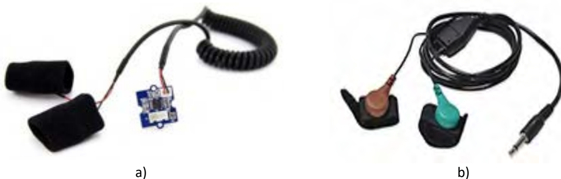
Figura 6. GSR (Galvanic Skin Response): a) Seeed Technology Co., Ltd., b) OBMS
