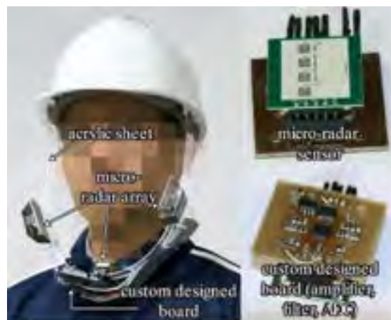
Figura12. Tongue-n-Cheek System (Università del Maryland) [41]
