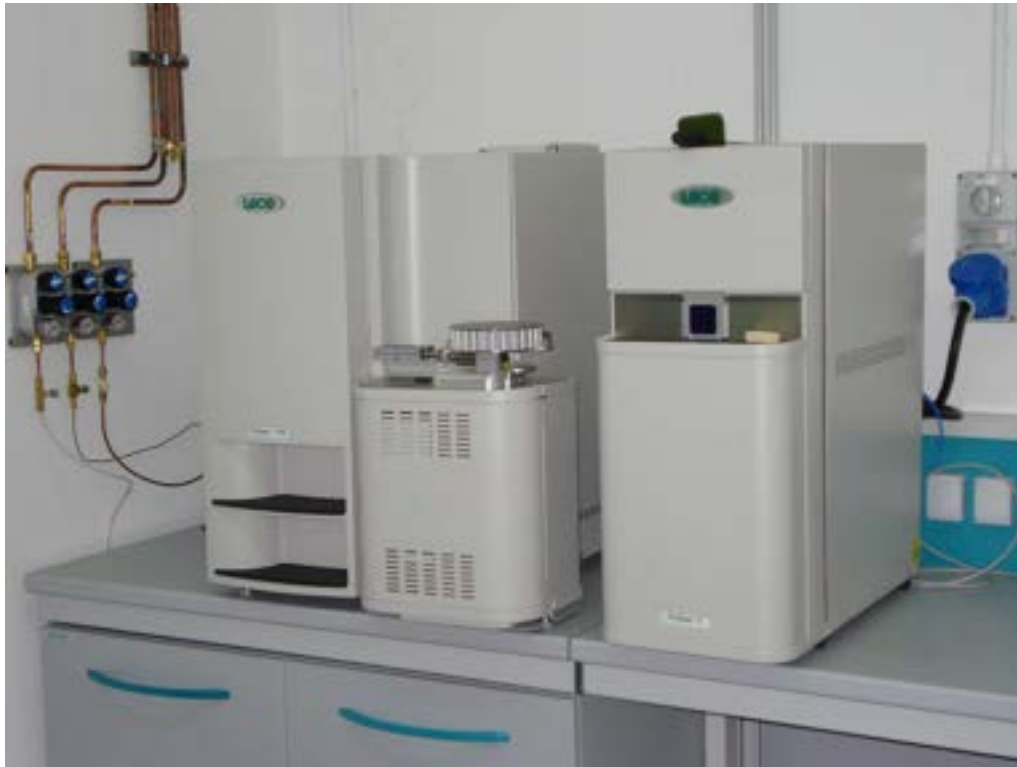
Fig. 5 – Determinatore CHN+S TruSpec Leco
