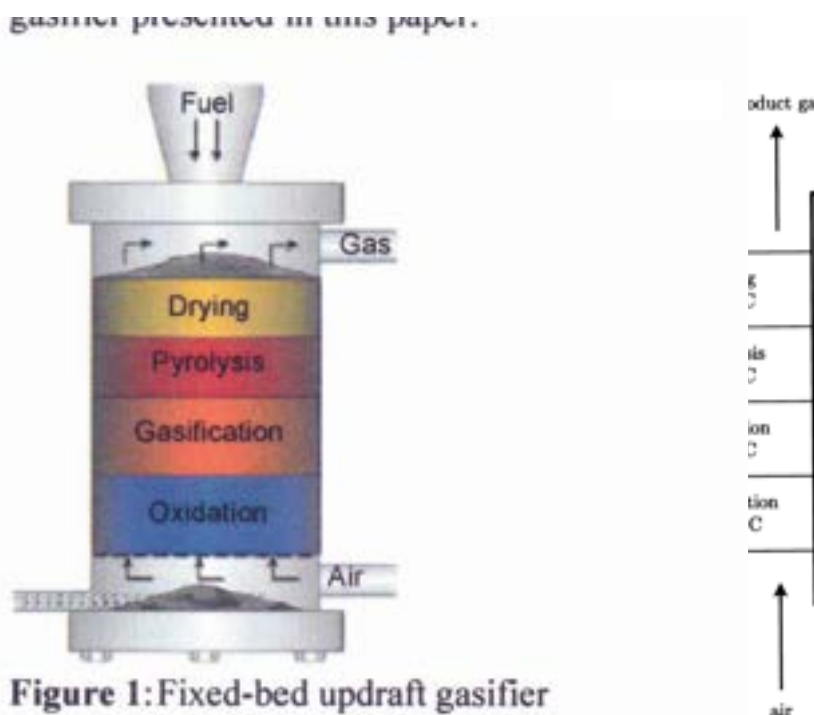
The fuel (pellets) is fed continuously from the top of the gasifier. The air is fed from the bottom. The product gas exits from the top of the gasifier.
