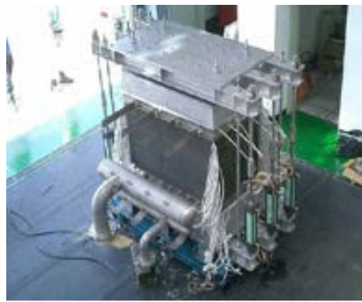
Figure A3 b. Internal manifolding configuration (courtesy of KEPRI)
