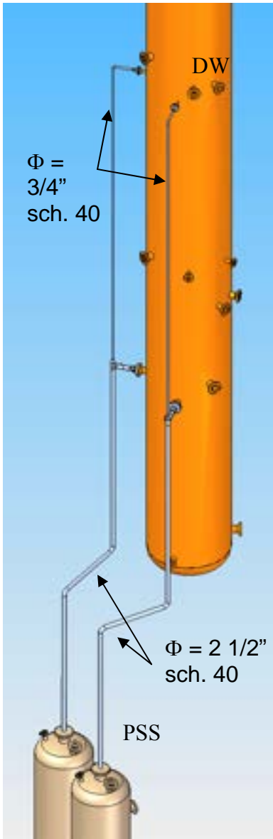
Fig. 12: Dry well connection to pressure suppression system
